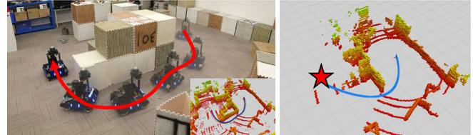
(a) Navigate in an aggressive manner in the original occupancy map. The vehicle plans a turn early and only replans after indeed observe the side wall.
