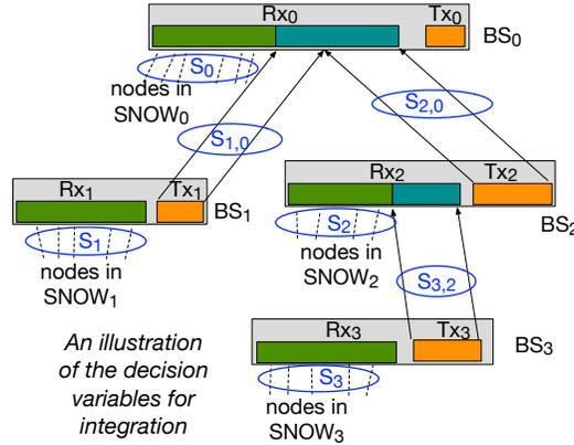
Figure 4.4: Integration using BS dual-radios.
