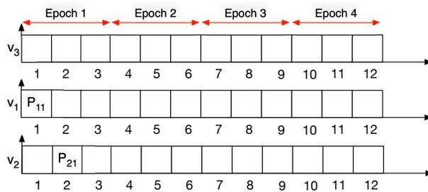
Figure 3.4: Example of Packet Scheduling in DistributedHART
