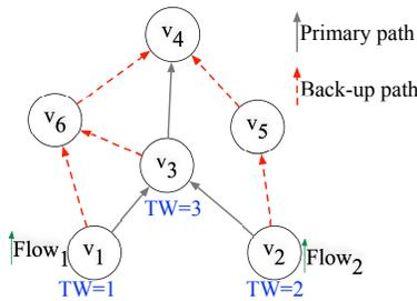
Figure 3.3: Example of Time Window Allocation in DistributedHART
