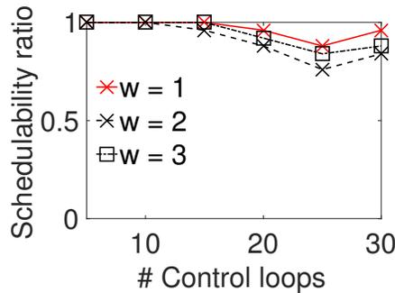
Figure 3.16: Schedulability ratio under Varying Window Lengths
