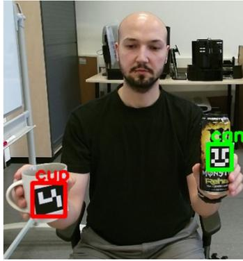
Figure 2: Clipped sample image of the object recognition visualization. The left marker is not tracked and therefore red. The right marker is currently tracked by the robot, which is indicated by a green bounding box. The learned label by the robot of each marker is written above the bounding boxes.
