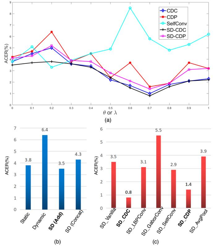
Fig. 9: Ablation study of CDC, CDP and static-dynamic representation. (a) Impact of  $\theta$  and  $\lambda$  in CDN. (b) Impact of dynamic representation. (c) Comparison among various convolutions and pooling. ‘SD’ is short for static-dynamic representation. Lower ACER indicates better performance.
