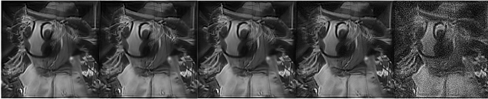
Fig. 5. In an experiment TIP4AW is used to estimate the original object from sets of input images with different noise levels. White Gaussian noise with varying standard deviations, \sigma = 10^{-5}, 10^{-4}, 10^{-3}, 10^{-2}, 10^{-1} , is added to the images. The estimated object corresponding to the sets of input images with different noise levels are depicted in this figure respectively. The quality in SSIM of the estimated objects can be found in Fig. 4.
