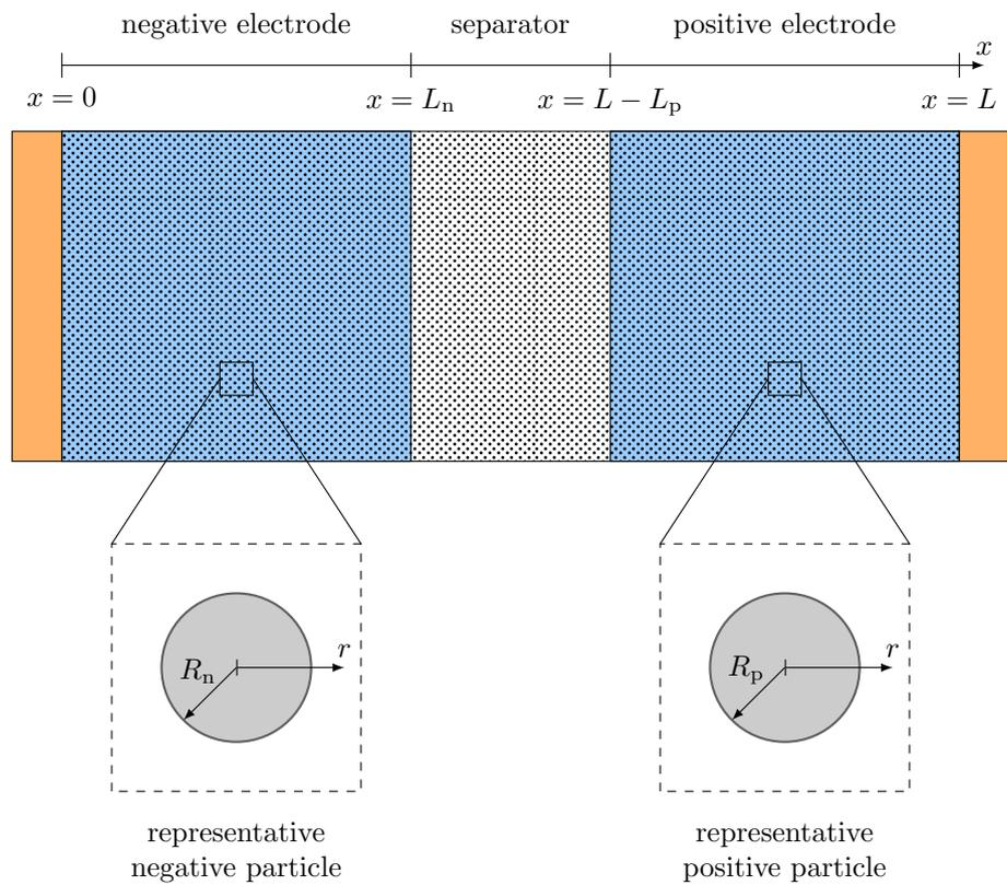
Figure 4: Geometry of the TSPMe. Note that we do not pose a geometry for the thermal model because it is a lumped model and therefore there is no space distribution for temperature. The subscripts n and p denote the parameters for the negative and positive electrodes, respectively.
