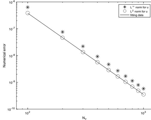
Figure 2: The discrete  $\ell^2$  and  $\ell^\infty$  numerical errors vs. temporal resolution  $N_T$  for  $N_T = 100 : 100 : 1000$ , with a spatial resolution  $N = 192$ . The surface diffusion parameter is taken to be  $\varepsilon = 0.05$ . The data lie roughly on curves  $CN_T^{-3}$ , for appropriate choices of  $C$ , confirming the full third-order accuracy of the scheme.
