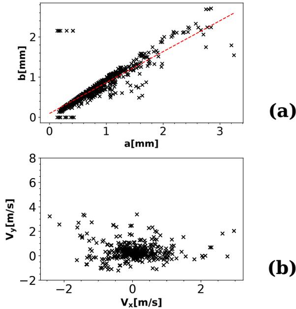
Fig. 17. (a) Droplet size characterization where  $a$  is the major-axis and  $b$  is the minor-axis of the droplet respectively in mm (b) Droplet velocity characterization showing both the  $x$  component velocity and the  $y$  component velocity.
