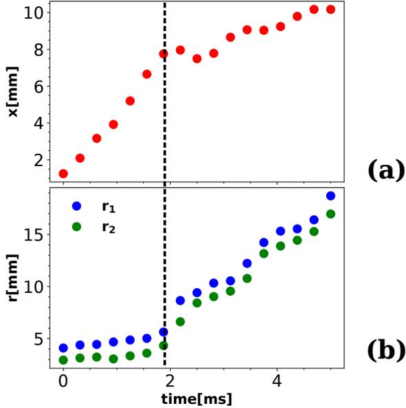
**Fig. 4.** Air puff characterization. (a) displacement of the leading vortex vs time in ms, (b) radial expansion of the leading vortex vs time in ms, showing both outer diameter and inner diameter of the leading vortex.
