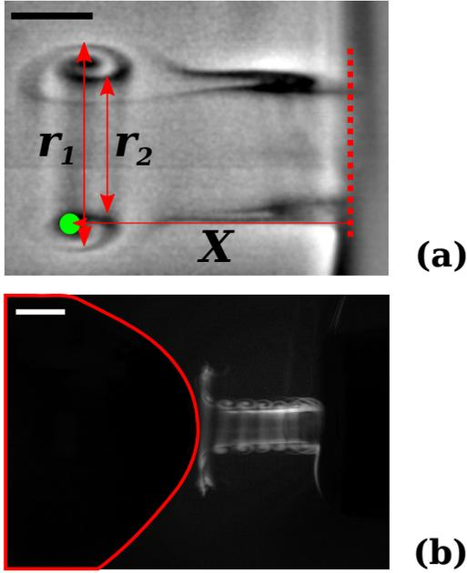
**Fig. 3.** Air puff characterization. (a) shows the smoke flow visualization of the leading vortex and the trailing jet along with the tracking parameters. The scale bar denotes 3mm in actual length, (b) depicts the propagation of the leading vortex towards a goat eye. The scale bar denotes 6mm in actual length.
