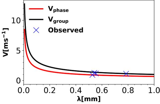
Fig. 9. Theoretical phase velocity and group velocity as a function of wavelength along with the experimental velocities.
