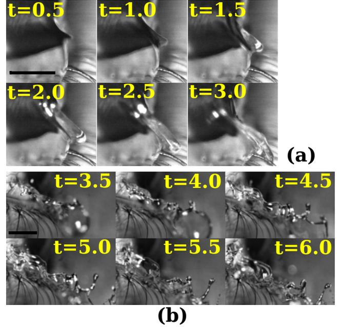
Fig. 11. Time sequence of the sheet expansion (a) denotes the initial sheet ejection, (b) denotes later sheet expansion. The scale bar is 3mm.
