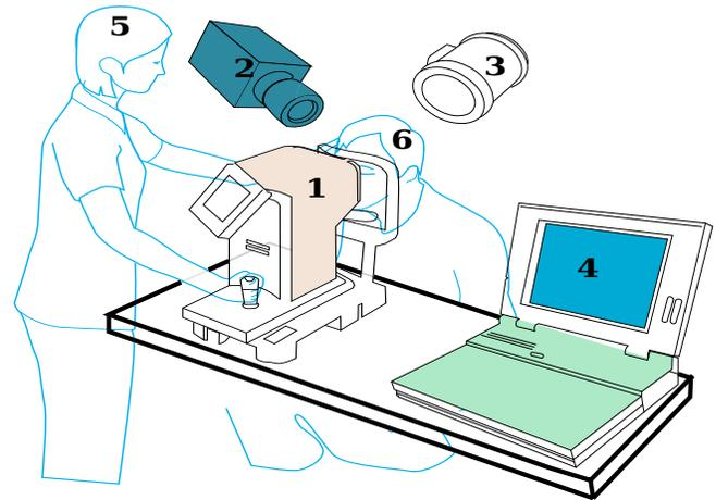
**Fig. 2.** Schematic of the experimental setup. The different components of the setup are 1: Non Contact Tonometer, 2: High Speed Camera, 3: Light Source, 4: Computer, 5: Tonometer Operator, 6: Human Subject
