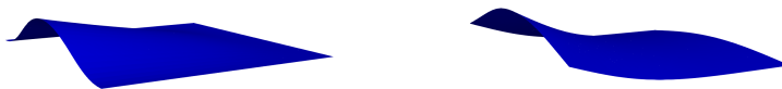
FIGURE 1. A trapezoidal-like plate is glued at the three edges of a square of unit size and is free at the remaining side, as suggested in [17] (left). For s small, the plate cannot sustain the in-plane compression and buckles up. The deformation \mathbf{y}(x_1, x_2) = (x_1, x_2, x_1^2(1-x_1)^2x_2^2)^T mimics this configuration and yields a target metric g = \mathbb{I}[\mathbf{y}] ; \mathbf{y} and g are thus compatible. Upon freeing the boundary conditions, the plate changes shape to a non-flat configuration with the same metric (right).
