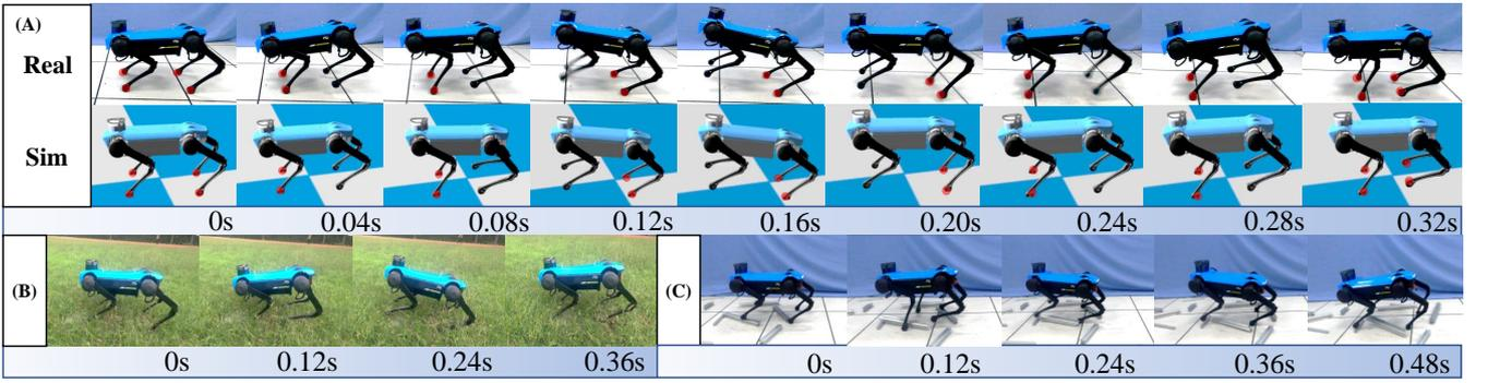
**FIGURE 2** Quadruped bounding in simulation and in the indoor and outdoor environments. (A) The comparison between simulation and real world implementation, red dots highlight the contact points with the ground. (B) and (C) Traversal over rough grass field and plastic floor with sparse obstacles.
