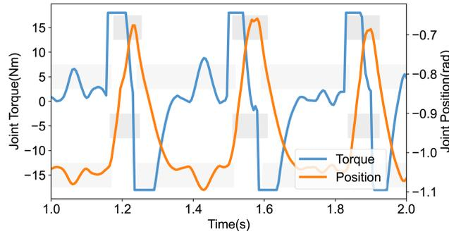
**FIGURE 9** Smooth joint position and torque during bounding and gray shades are the estimated contact states.
