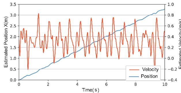
**FIGURE 10** Position and forward velocity of the robot torso.
