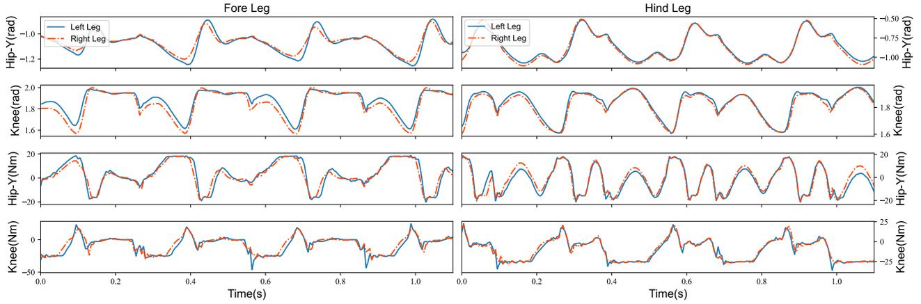
**FIGURE 4** Experimental data of joint positions and torques during bounding, showing the symmetry between left and right legs.
