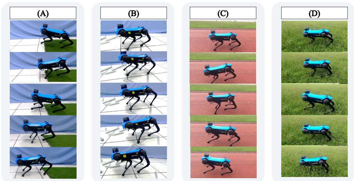
**FIGURE 8** Jueying Mini robot bounding in various testing scenarios using the same PF-DRL trained policy. (A) Smooth transitions between regions with different properties (friction, stiffness). (B) Restoring balance after stepping on slippery objects twice. (C) Traversing soft outdoor ground. (D) Robust traversal on uneven grass field with shallow pits.
