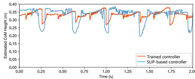
**FIGURE 12** Height of CoM from the robot state estimation.
