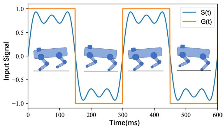
**FIGURE 3** Illustration of contact states and reward.  $G(i, t)$  represents current contact state of the robot and  $S(t)$  indicates whether that foot should touch the ground. The plot shows example signals of forelimbs when bounding with a period of 0.3s, and an illustration of an ideal case of the robot in motion in order to achieve the maximum reward in the *Gait Reward* term.
