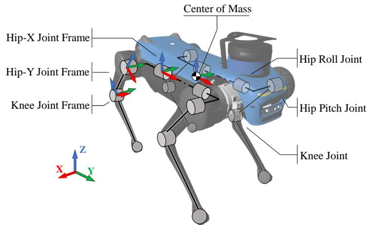
**FIGURE 5** Jueying Mini robot and its kinematic configuration.
