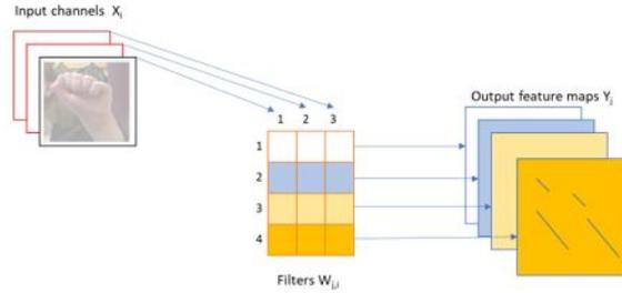
Figure 3: Fig. 3. Illustration of how the feature maps are computed, where  $W_{j,i}$  are the  $k \times k$  filters used on the input channels  $X_i$  to obtain output feature maps  $Y_j$
