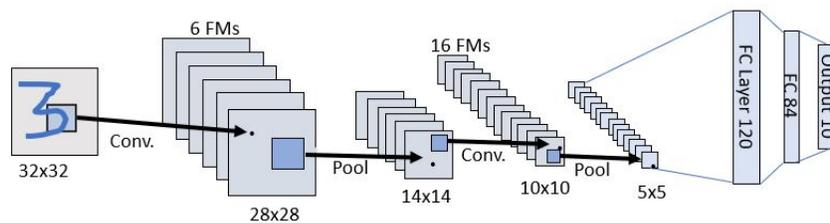
Figure 2: The LeNet-5 network and how it processes an input image via convolutions (Conv.) and pooling operations to produce features maps (FMs) and uses fully connected (FC) layers to perform classification
