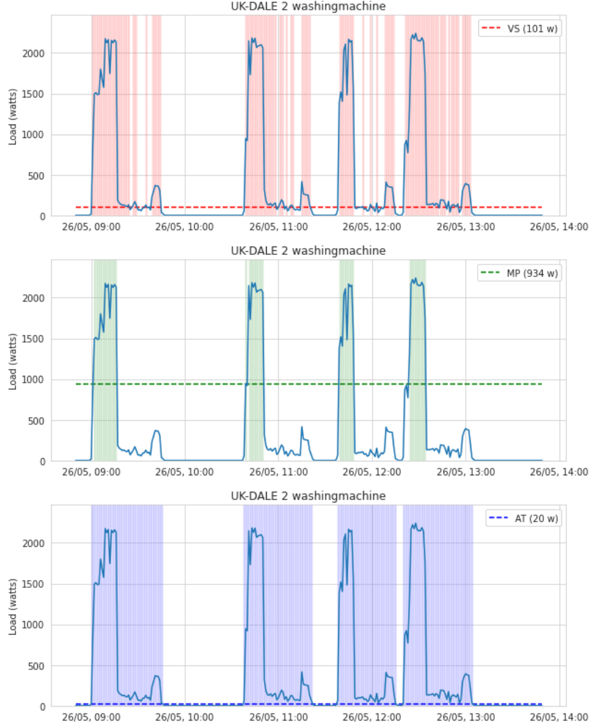
Figure 2: Sample from the washing machine power load sequence, depicting how different thresholding methods classify each instance as ON or OFF.
