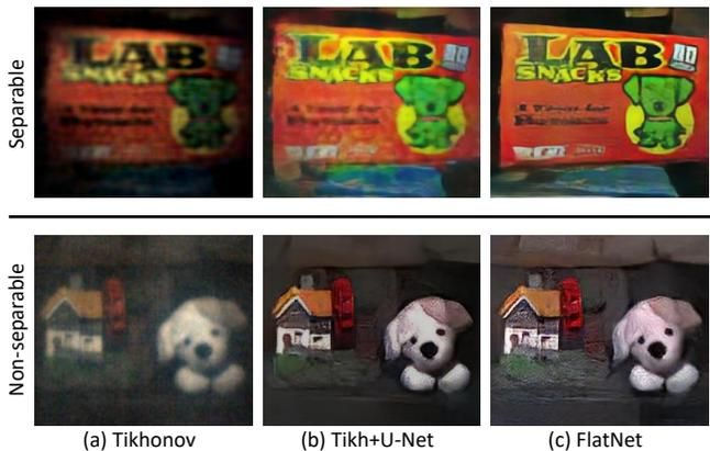
Fig. 8. **Comparison of FlatNet with Tikh+U-Net.** Top row shows the comparison of FlatNet-sep with Tikh+U-Net while the bottom row shows the comparison of FlatNet-gen with Tikh+U-Net. FlatNet provides sharper and more photorealistic reconstructions compared to Tikh+U-Net for both separable and non-separable models.
