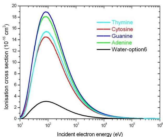
Figure 6 : Total ionisation cross sections for the DNA bases and water.
