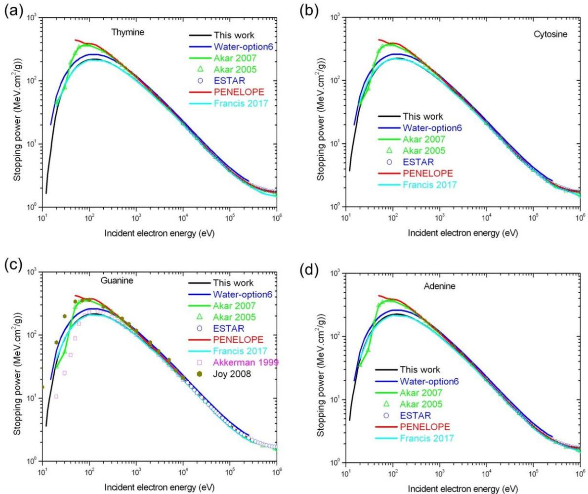
Figure 10: Stopping power of the four nucleobases for electrons ranging from 11 eV - 1 MeV as calculated in this work in comparison with Geant4-DNA water-option6 simulation and other results from the literature [20, 61-65]. Stopping power in the four nucleobases was derived from the input material data file of PENELOPE code.
