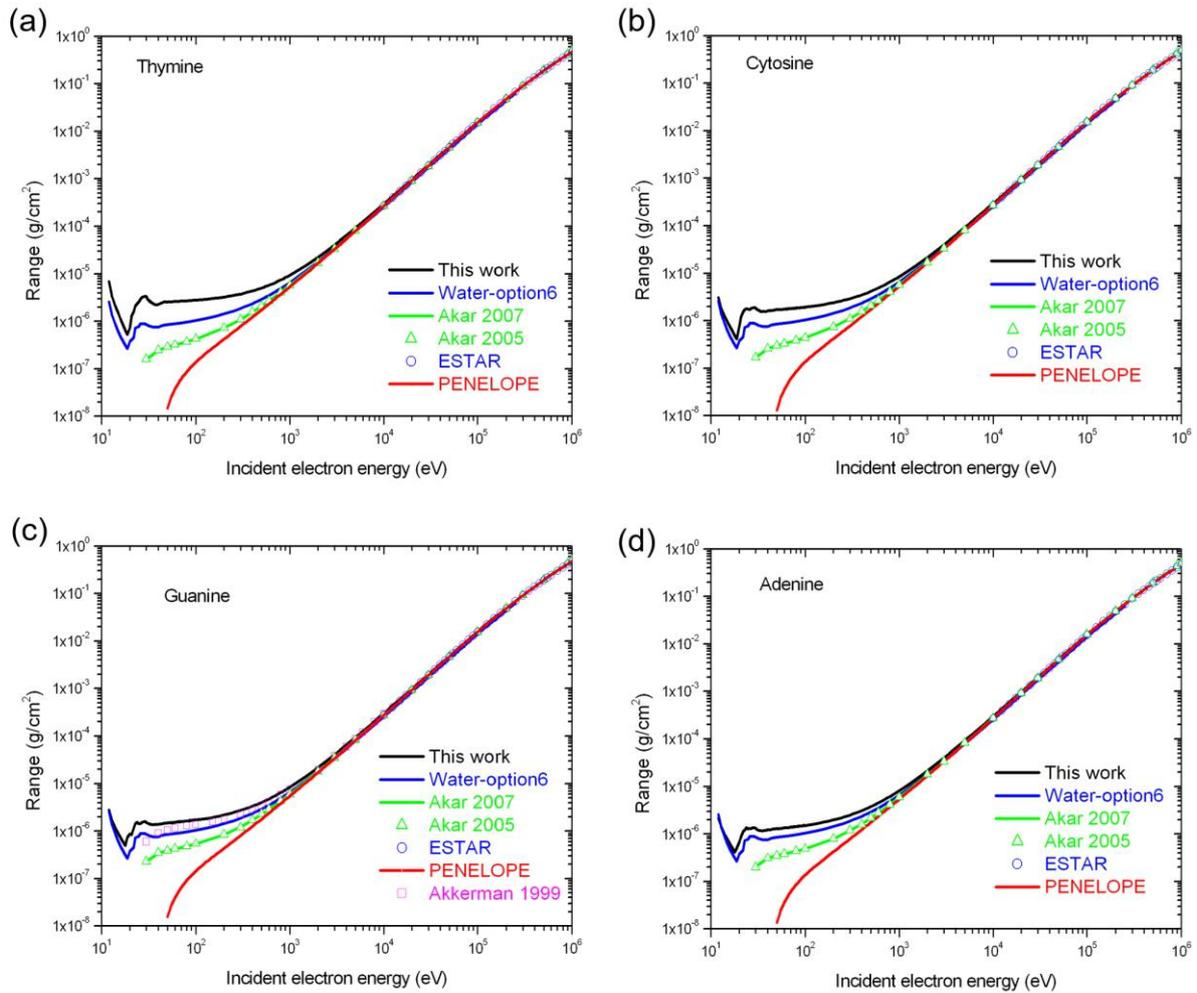
Figure 11: Range of electrons ranging from 11 eV - 1 MeV in the four nucleobases as calculated in this work in comparison with Geant4-DNA water-option6 simulation and other results from the literature [61, 63-65]. Range in the four nucleobases was derived from the input material data file of PENELOPE code.
