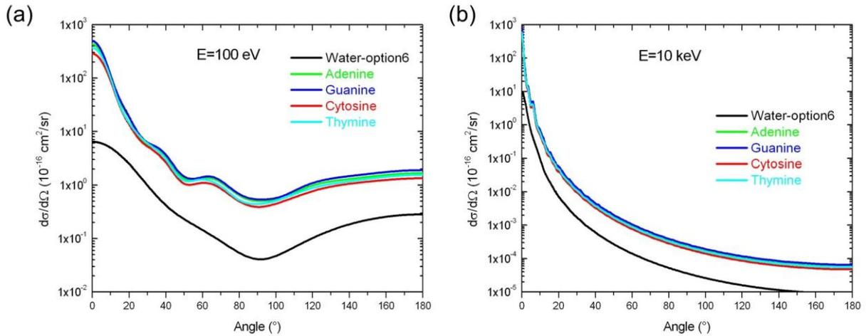
Figure 1 : Elastic differential cross section for 100 eV (a) and 10 keV (b) electron collisions with adenine, guanine, cytosine, thymine and water respectively
