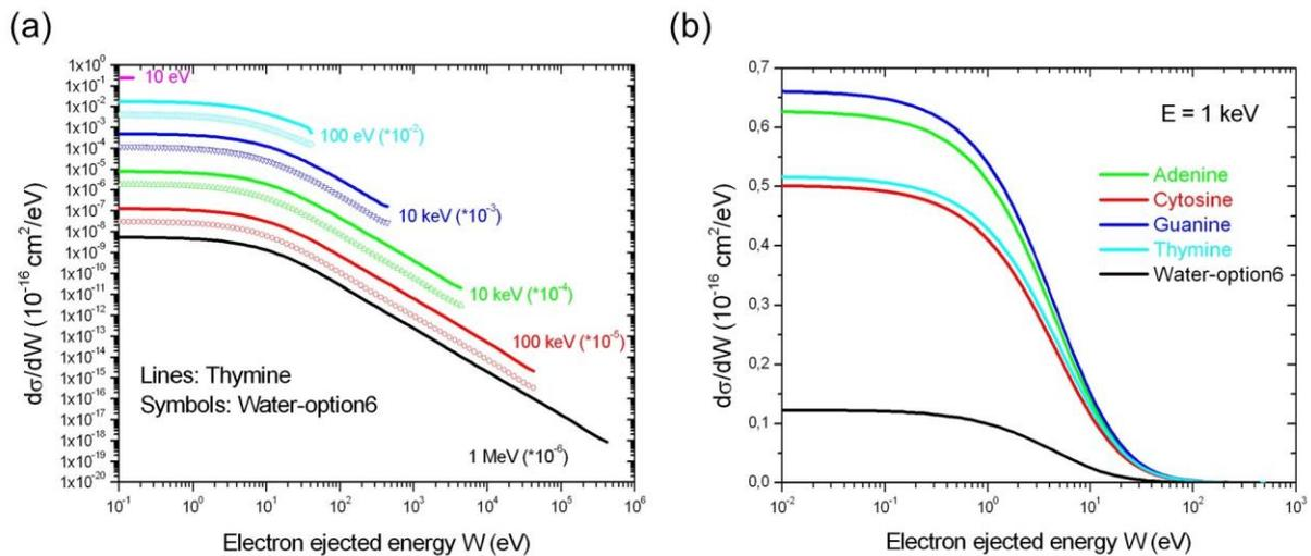
Figure 8 : Differential cross sections by electrons as a function of the electron ejected energy in thymine and in water at different incident electron energies(a), and in the four bases and water at 1keV incident electron energy (b).
