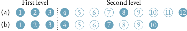
Fig. 1: 2-level nested array with N_1 = N_2 = 3 and d = 1 . (a) Conventional design: L = N_1 + 1 , does not enable LS-based blind calibration. (b) Proposed design: L = N_1 , enables LS-based blind calibration. Filled bullets represent sensors, while empty bullets represent spaces (absence of a sensor).
