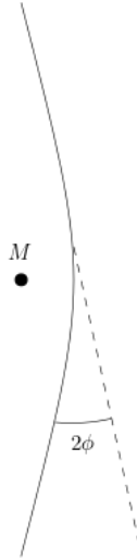
FIGURE 1.1: Bending of light by the Sun. In Newtonian mechanics, the photon is assumed to follow an hyperbola.
