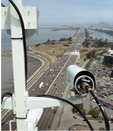
Figure 2 Recording of vehicle trajectories using a digital video camera overlooking a highway (Halkias and Colyar, 2006).
