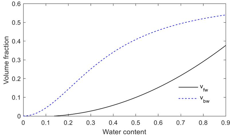
Figure 2 Variation of volume fractions of free water and bound water with respect to gravimetric water content  $m_g$ .
