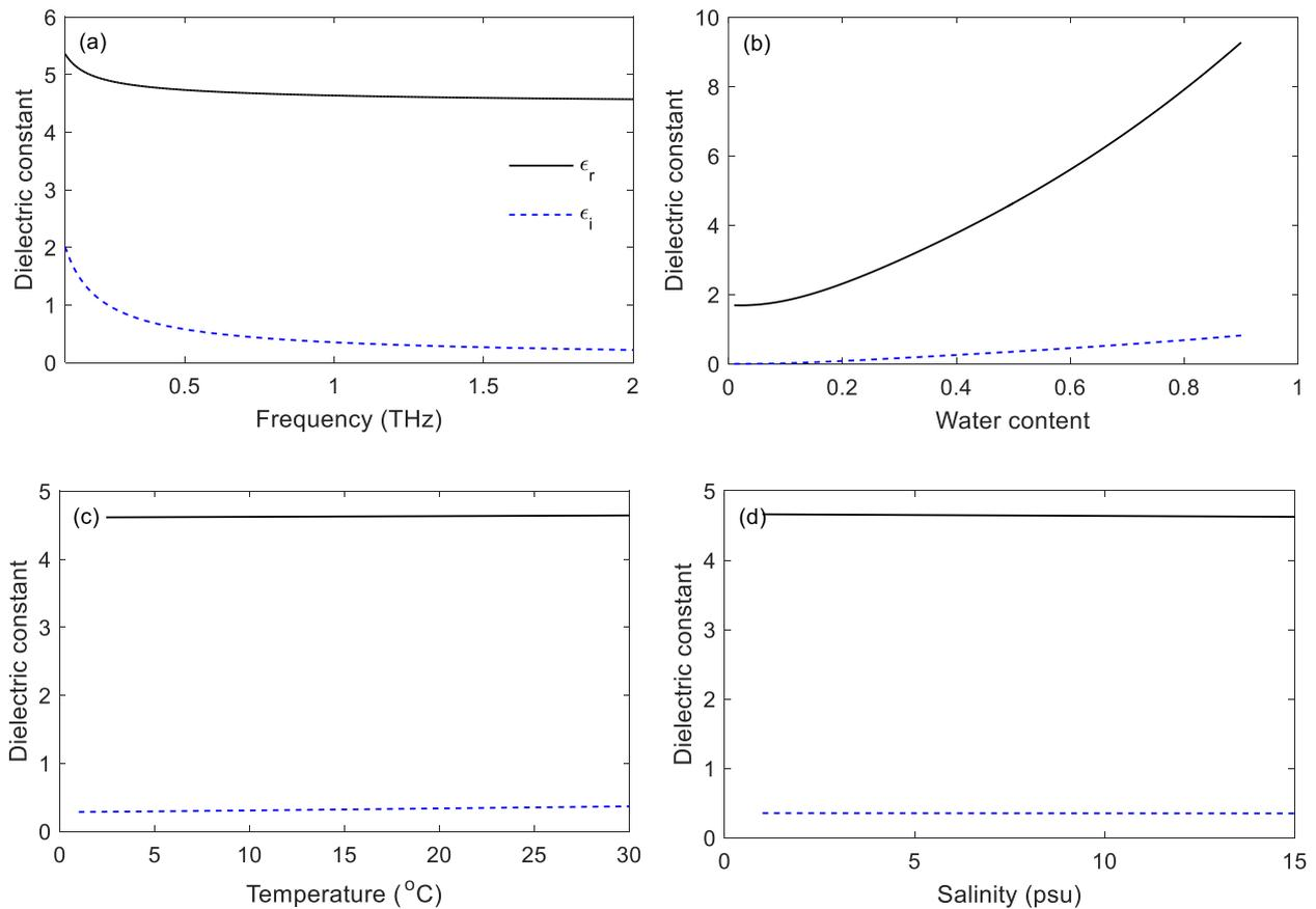
Figure 4 (a) Dielectric spectrum of a fresh leaf with water content  $m_g = 0.5$ , temperature  $T = 25^\circ\text{C}$  and salinity  $S = 10$  psu; (b) Evolution of dielectric constant with respect to water content with frequency at 1 THz, temperature  $T = 25^\circ\text{C}$  and salinity  $S = 10$  psu; Variation of dielectric constant of plant leaves
