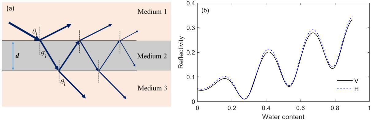
Figure 5 (a) Three-layered structure with planar boundaries; (b) Variation of reflectivity by plant leaves with respect to water content with a THz frequency at 1 THz, water content  $m_g = 0.5$ , salinity  $S = 10$  psu, temperature  $T = 25^\circ\text{C}$  and leaf thickness  $d = 0.27\text{mm}$ .
