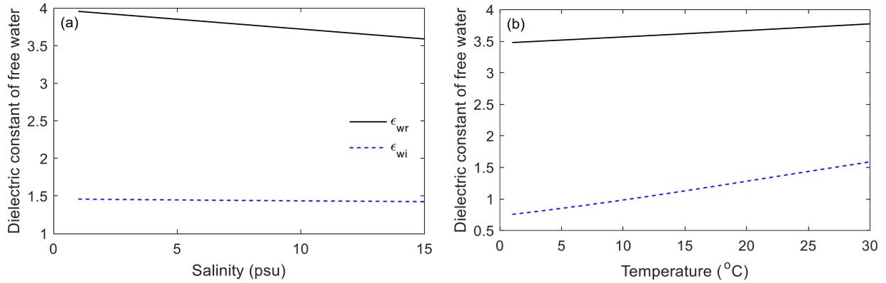
Figure 3 Variation of dielectric constant of free water with respect to (a) salinity and (b) temperature with THz frequency at 1 THz, water content  $m_g = 0.5$ , salinity  $S = 10$  psu and temperature  $T = 25^\circ\text{C}$ .
