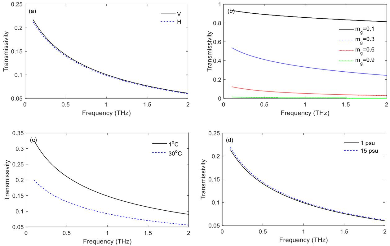
Figure 8 Variation of THz transmissivity with respect to frequency under different (a) polarization, (b) water content, (c) temperature and (d) salinity. Incidence angle  $\theta_i = 10^\circ$ , water content  $m_g = 0.5$ , temperature  $T = 25^\circ\text{C}$ , salinity  $S = 10$  psu, leaf thickness  $d = 0.27\text{mm}$ .
