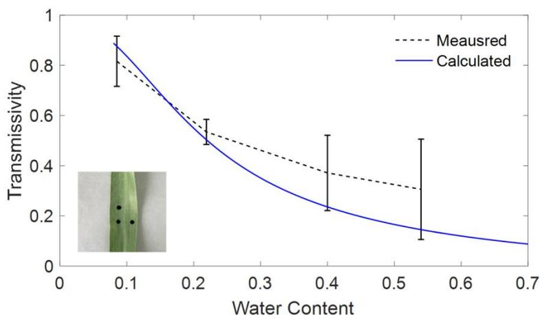
Figure 9 Measured and calculated THz transmissivity versus water content with incidence angle  $\theta_i = 0$ , temperature  $T = 25^\circ\text{C}$ , salinity  $S = 10$  psu and leaf thickness  $d = 0.27\text{mm}$ . The vertical error bars with 95 % confidence interval shown in the plot represent the standard deviation of recorded data. The insert shows a leaf sample we used with three black dots representing the measured positions.
