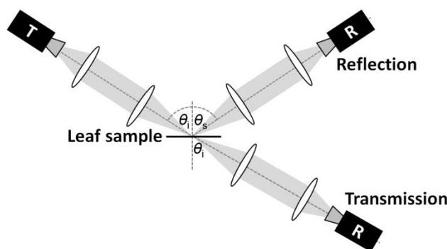
Figure 1 Basic reflection and transmission geometries for THz monitoring technique.
