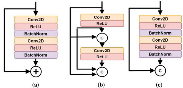
FIGURE 5. (a) Residual block (b) Dense block (c) ResDense Block
