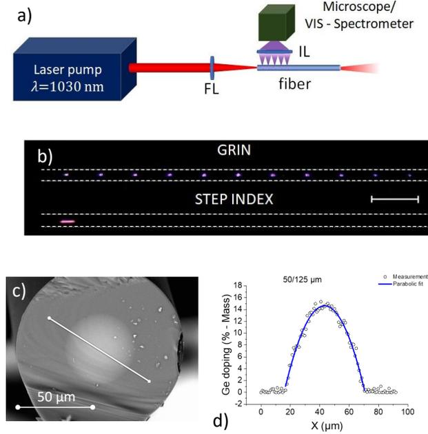
Figure 1: (a) Schematic of the experimental setup. (b) Microscope image of luminescence scattered from either GRIN or step-index fibers. Dashed lines stand for the cladding-air interface, while the scale bar corresponds to 1 mm. (c) SEM image of a GRIN fiber section. (d) % mass Germanium concentration in the Ge-doped GRIN fiber.
