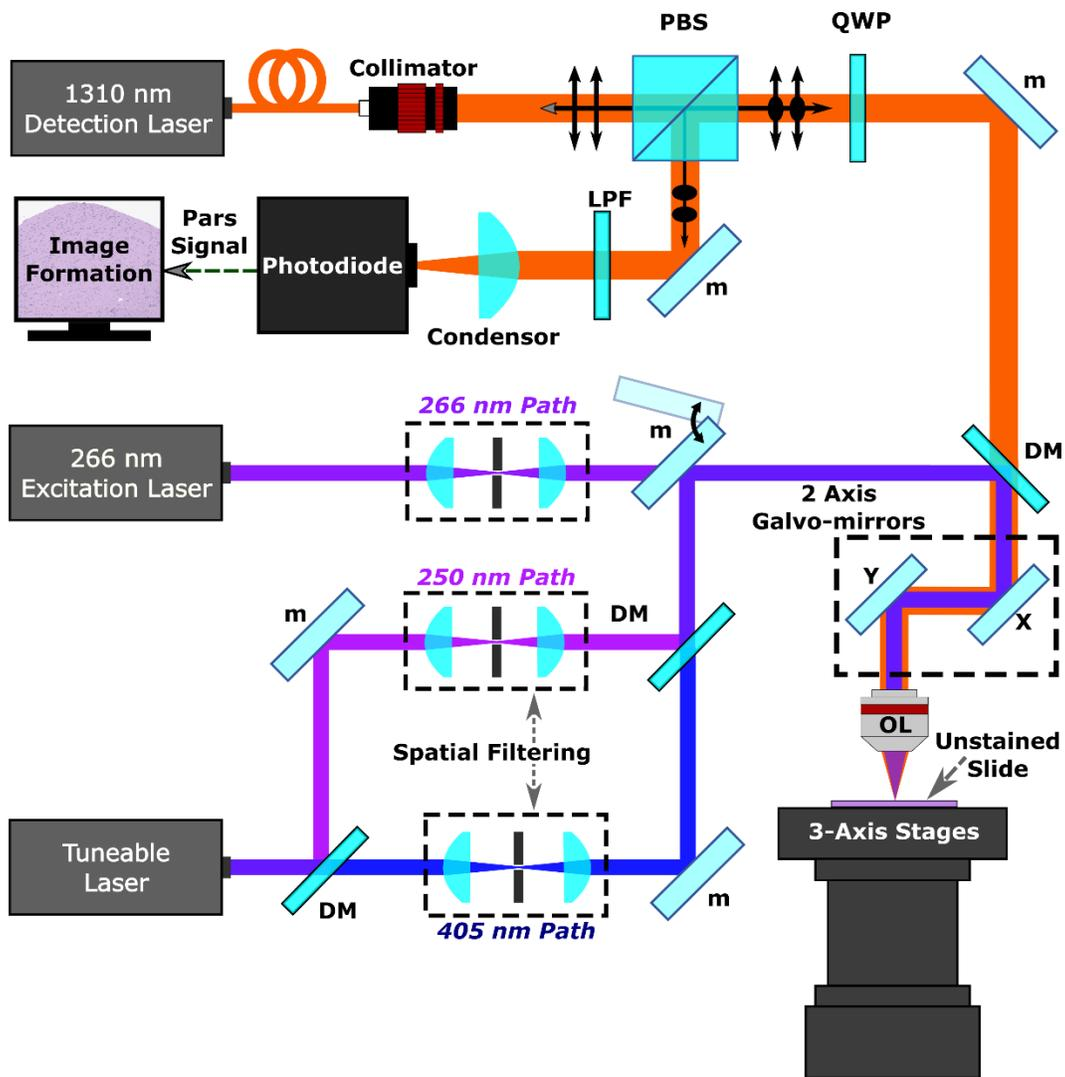
**Figure 1:** Simplified Schematic of the PARS system. Component labels are defined as follows: polarizing beam splitter (PBS), long-pass filter (LPF), quarter-wave plate (QWP), objective lens (OL), dichroic mirror (DM), fold mirror (m).
