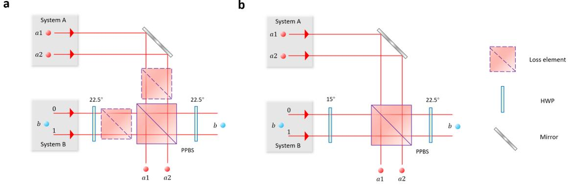
Fig. S3.  $CX_4$  gate with linear optics. **a**, The standard optical  $CX_4$  gate. **b**, The simplified optical  $CX_4$  gate.
