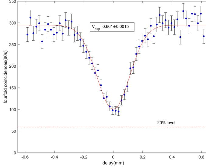
Fig. S2. HOM interference at the PPBS for a  $|HH\rangle$  input. In case of perfect interference, the count rate should drop down to 20%, leading to a theoretically achievable dip visibility of 80%.
