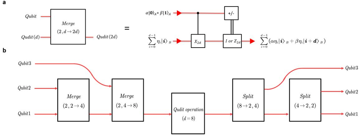
Fig. S5. **a**, The Merge operation. The quantum circuit for merging the quantum information of a qubit and a d-dimensional qudit into a 2d-dimensional qudit. **b**, Implementing a three-qubit quantum gate.
