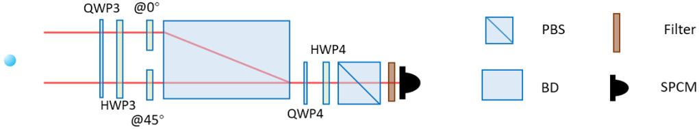
Fig. S4. State analyzer for a single-photon ququart state with both polarization and spatial degrees of freedom.
