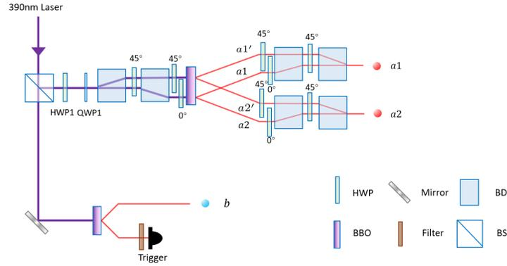
Fig. S1. Experimental setup for generating two photon pairs.
