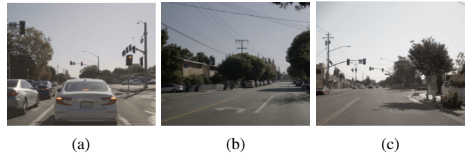
Fig. 1: Challenging urban scenarios for stop line detection: (a) Occlusion on stop line. (b) The stop line for cross-traffic on the left can easily be confused with a regular lane marking. (c) The stop line can barely be seen in the camera from a distance of around 30 meters.
