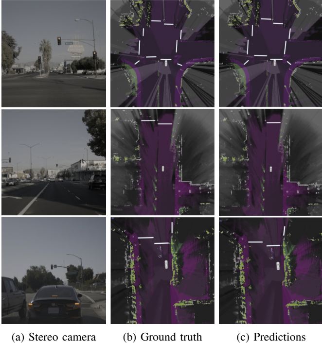
Fig. 6: Qualitative results of our stop line estimation approach. The front camera image is shown as reference (left). The results indicate that our approach is able to detect stop lines for all lanes (top), at high distances (middle), and during occlusion (bottom).
