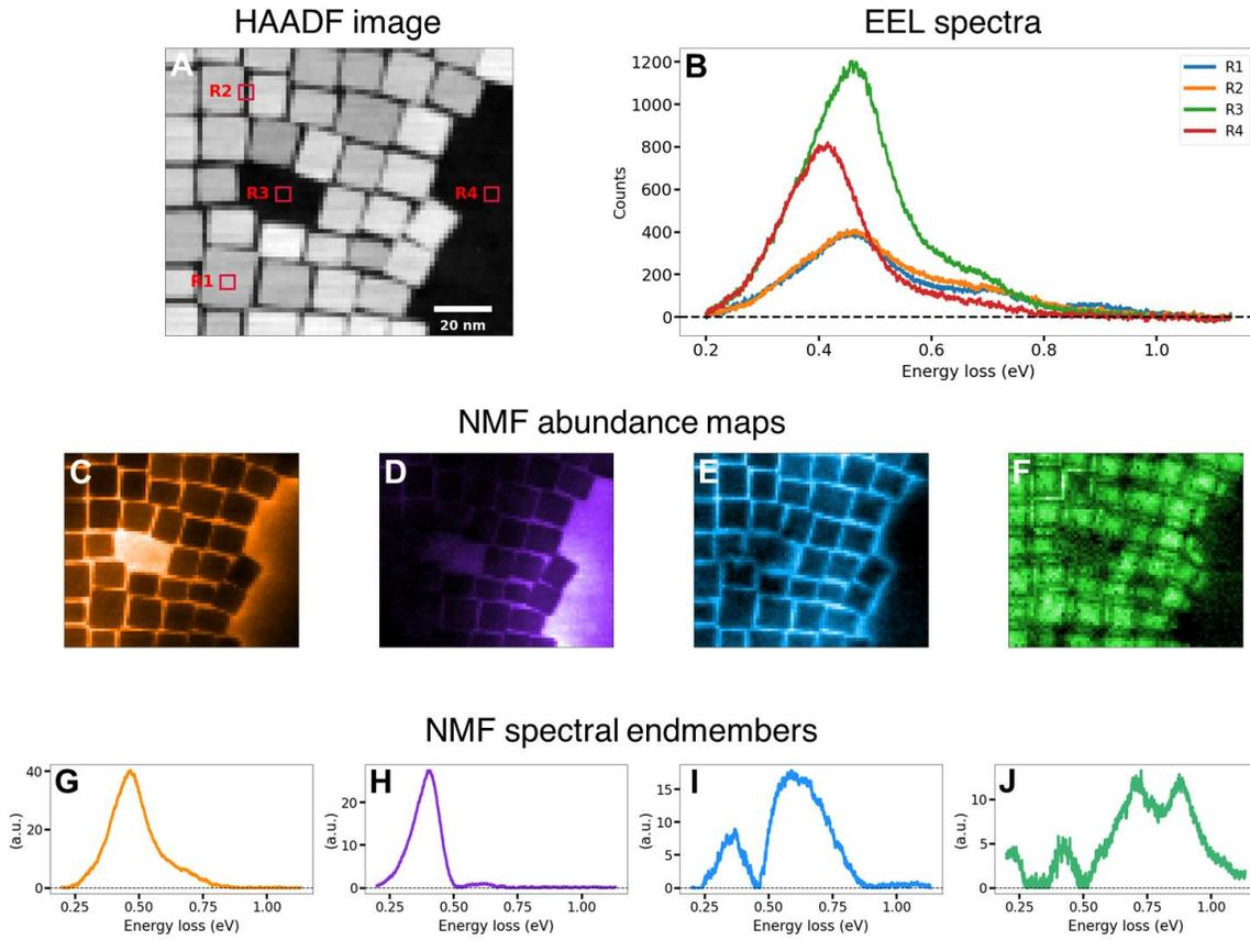
**Figure 1.** (a) HAADF-STEM image of nanoparticle array. (b) EEL spectra from selected locations (denoted by squares in (a)). (c-j) First four NMF components, (c-f) component abundance maps (g-j) component spectral endmembers.
