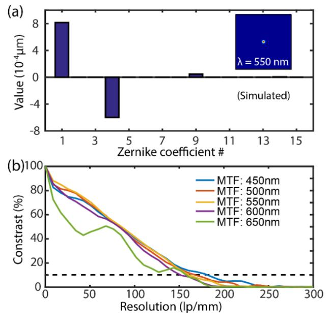
Fig. 3. (a) Aberrations analysis from simulated PSF at  $\lambda = 550 \text{ nm}$  (inset). (b) Experimental modulation-transfer-function (MTF). Resolution is  $175 \text{ lp/mm}$  at 10% contrast.
