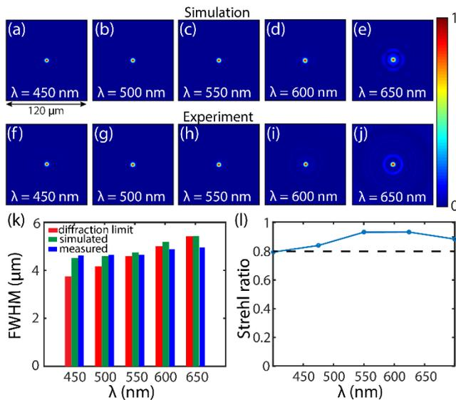
Fig. 2. (a-e) Simulated and (f-g) measured point-spread functions (PSFs) within the designed band: 450-650 nm. (k) Measured, simulated and diffraction-limited full-width at half maximum (FWHM) as a function of wavelength of an individual MDL. (l) Measured strehl ratio (SR) (wavelength averaged  $\text{SR} = 0.88$ ). A lens is considered diffraction limited when the  $\text{SR} > 0.8$ .
