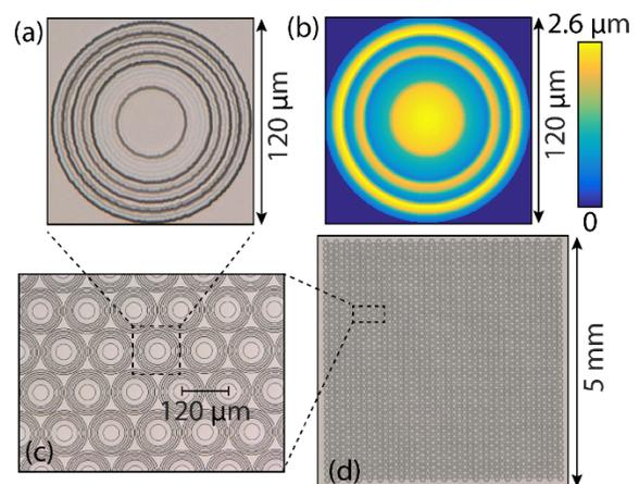
Fig. 1. (a) Optical micrograph of a single fabricated microlens and (b) its corresponding designed geometry. (c) Magnified image of a portion of the hexagonal-closed-packed microlens array with pitch = 120  $\mu\text{m}$ . (d) Image of the entire 40 x 40-microlens array. The size of the array is 5 mm, which is almost of the same size of the CMOS image sensor used in this study.
