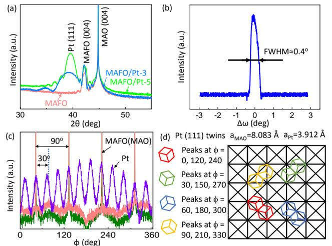
FIG. 1. XRD analysis of samples. (a) XRD  $2\theta/\omega$  scans of MAFO (13 nm)/Pt (5 nm), MAFO (13 nm)/Pt (3 nm), and MAFO (13 nm). (b) Rocking curve scan about the Pt (111) peak for the MAFO (13 nm)/Pt (5 nm) sample shown in (a), with  $\text{FWHM} \approx 0.4^\circ$ . (c) XRD  $\phi$  scans on the (113) plane of the MAFO (13 nm)/Pt (5 nm) sample. Pink: MAFO. Green: MAO. (d) Lattice matching relationship between the Pt and MAFO (MAO) unit cells.
