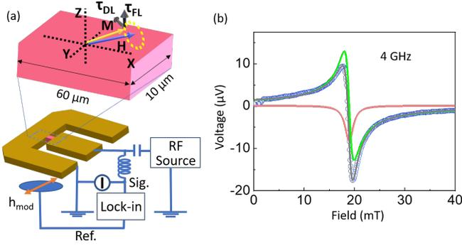
FIG. 2. ST-FMR measurement setup. (a) MAFO/Pt stack etched to a  $60 \mu\text{m} \times 10 \mu\text{m}$  strip. Magnetization, external field, rf field, and SOTs are shown as the arrows. The ground-signal-ground Au electrode connects MAFO/Pt to the external circuit. (b) FMR spectrum at 4 GHz. Red curve: symmetric Lorentzian contribution. Green curve: antisymmetric Lorentzian contribution. Blue curve: total fit.
