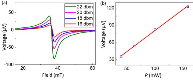
FIG. 7. (a) Exemplary ST-FMR spectra at different microwave powers. (b) ST-FMR amplitude vs. microwave power.
