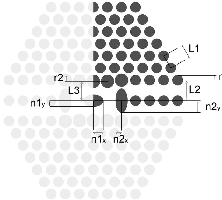
Figure S.5.1: Geometrical parameters for the dual-core waveguide segment
