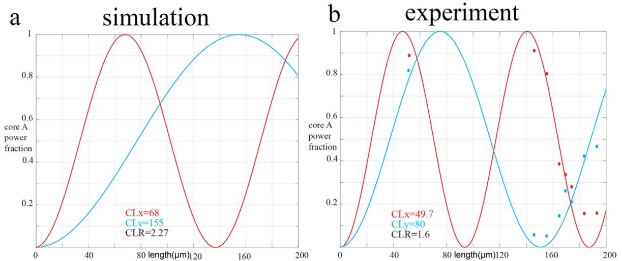
Figure S.5.2: **Simulations do not match experiments** a) Simulation of the power distribution among the cores for different lengths of the dual-core PCF segment for the starting design of our optimisation process. b) Experimental values and fitting of the coupling lengths on the same PCF geometry as 3D printed and integrated with the down-taper and fan-out sections
