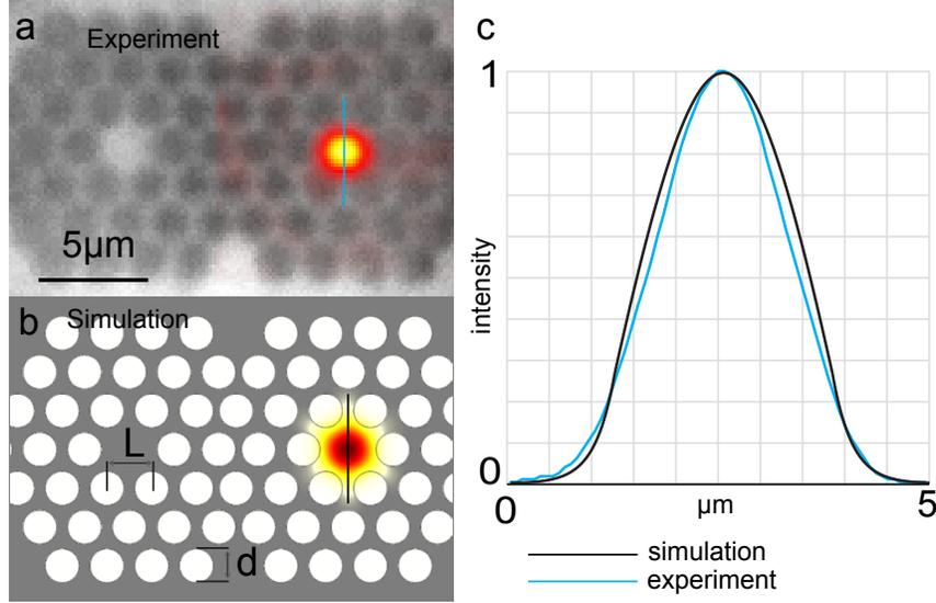
Figure S4: **Simulation and characterization of fan-out output mode at 1550 nm.** a) Optical image. b) Simulation. c) Intensity profiles of experiment and simulation. ( $d=1.5 \mu\text{m}$   $L=2 \mu\text{m}$ )
