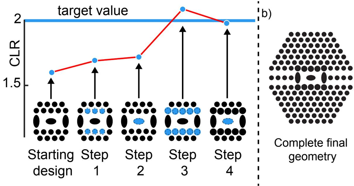
Figure 4: **Experimental optimisation of the PCF PBS geometry.** a) Progression of the best CLR in each step of the optimisation process towards  $\text{CLR} \rightarrow 2$ . The geometrical elements that have been changed in each iteration step are highlighted in blue (only the important central holes are displayed); b) Complete cross-sectional PCF geometry of the optimised PCF PBS design.
