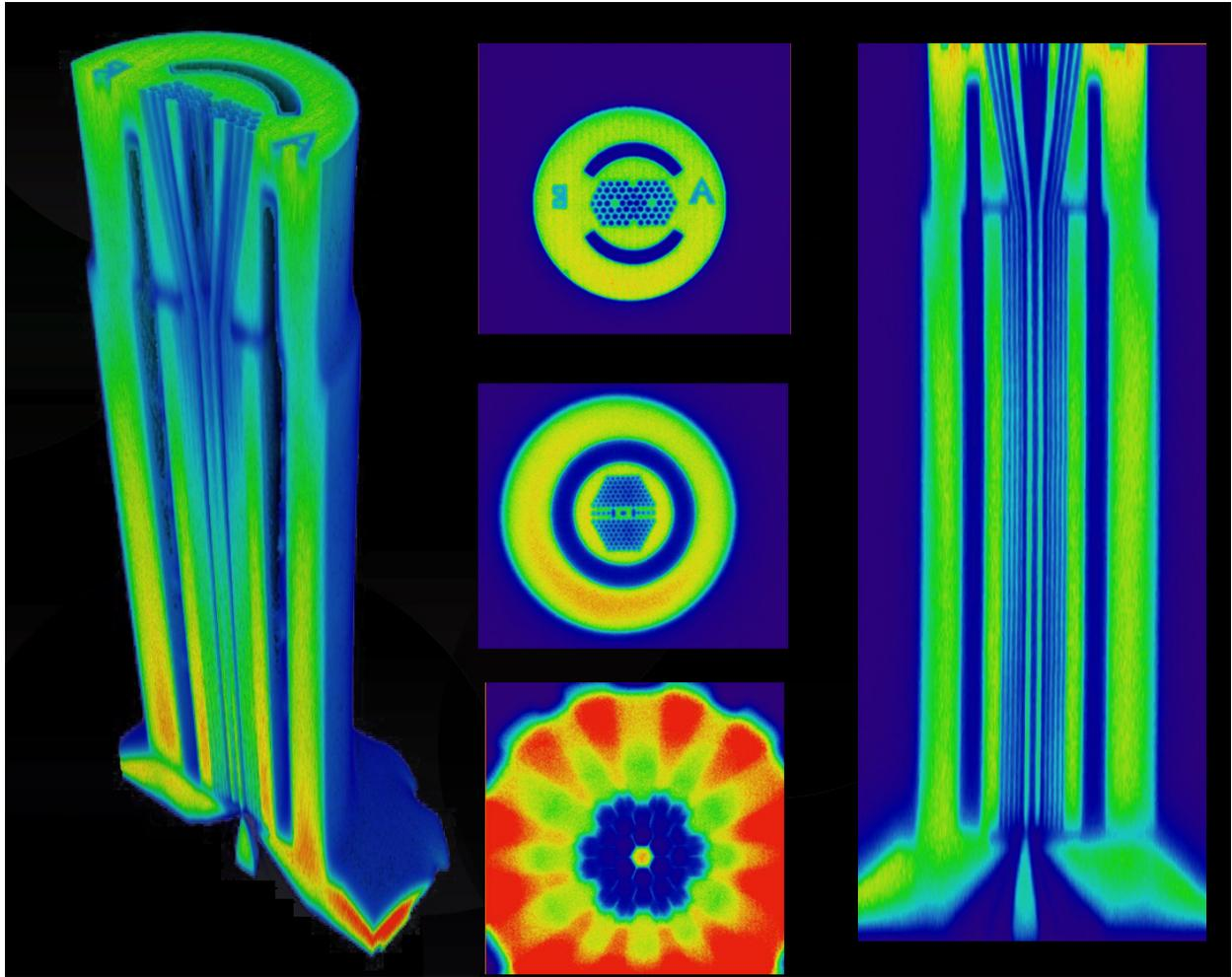
Figure S.8: Rendered three dimensional stack and cross-sections obtained with confocal fluorescence microscopy of one complete PCF PBS structure
