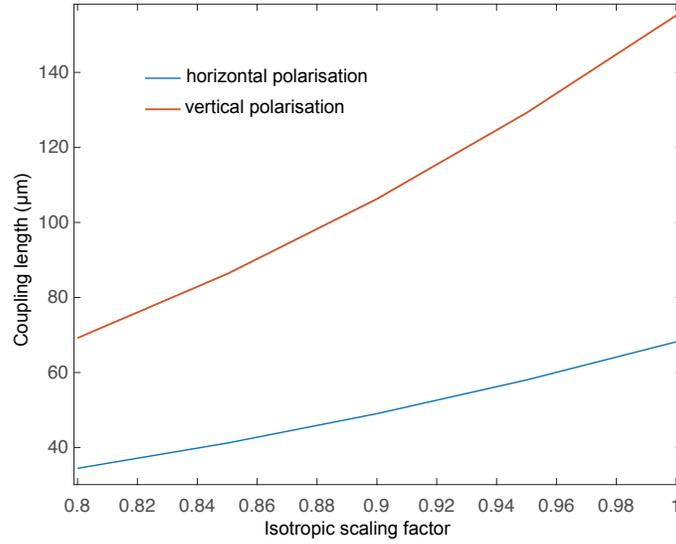
Figure S.5.3: **Simulations of the effect of isotropic shrinkage on the coupling lengths of the dual-core directional coupler.** We simulated the effect of an isotropic scaling of the dual-core section geometry on the coupling lengths at 1550 nm. The shrinkage leads to a significant reduction of the coupling lengths, in line with the observed difference between simulations and experiments (see Figure S.5.2).
