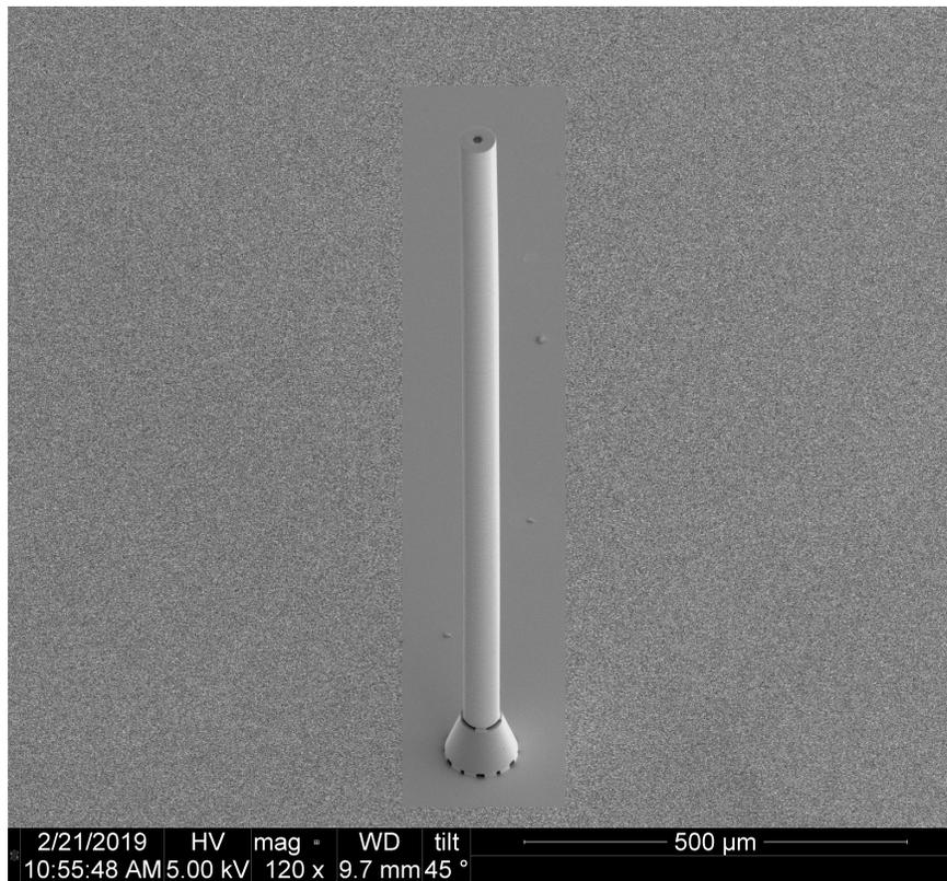
Figure S1: Full length scanning electron micrograph of the 1 mm-long 3D printed HNL PCF-like segment reported in Fig. 1a
