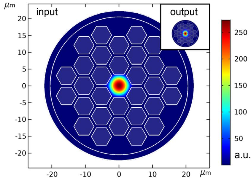
Figure S3: **Design of the down-taper segment.** We show the input and output cross-sections of the down-taper segment, along with the fundamental modes at 1550 nm at each section, as calculated with modal analysis (COMSOL). The figures are at the same scale.
