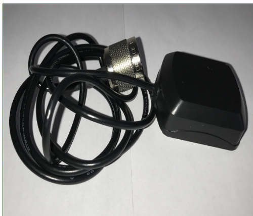
Figure 5. RF GPS Only Passive Patch Antenna
