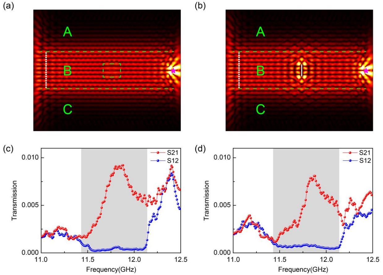
Fig. 4. (a),(b) Simulated electric field intensity distributions at 11.9 GHz in the heterostructures with a void defect, in which 10 unit cells are removed inside the green dashed rectangle and a PEC obstacle, respectively. (c),(d) Measured average transmission spectra S21 and S12 in domain B for the void and PEC defects, respectively.
