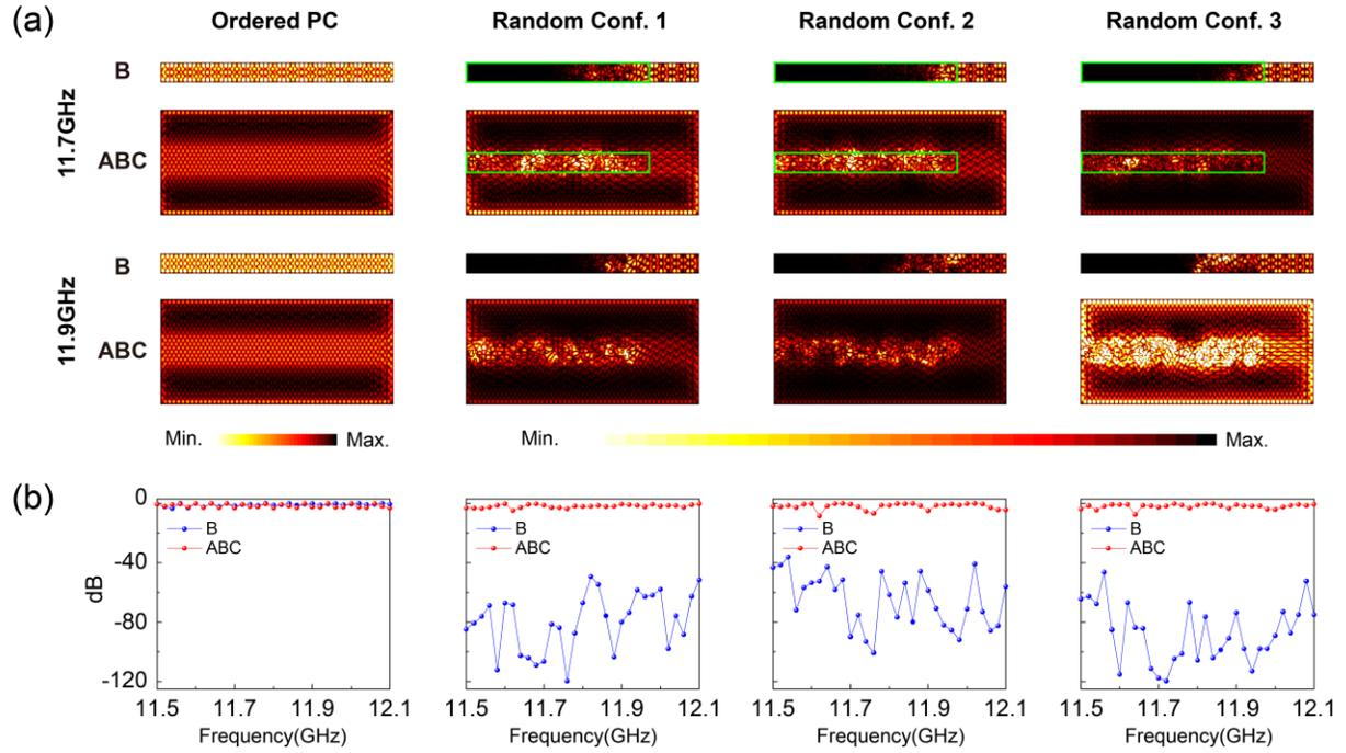
FIG. 5. (a) The simulations of a crystal  $B_5$  and heterostructures  $A|B_5|C$  in the ordered PC and three different configurations of random PCs, in which the permittivity of YIG rods inside the green rectangle is randomly selected between 1 and 26.6. Electromagnetic waves are incident from the right. (b) The corresponding transmission spectra for  $B_5$  and heterostructures  $A|B_5|C$ .
