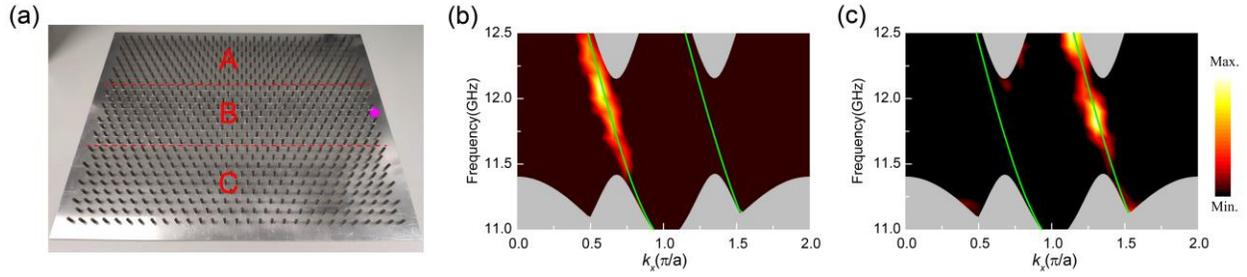
Fig. 2. (a) The photo of the A|B<sub>9</sub>|C sample. The magenta star marks the position of the point source. (b),(c) The selective excitations of the even (b) and odd (c) TOLWSs by the corresponding point dipolar sources.
