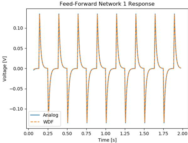
Figure 5: WDF simulation results compared to the analog reference.
