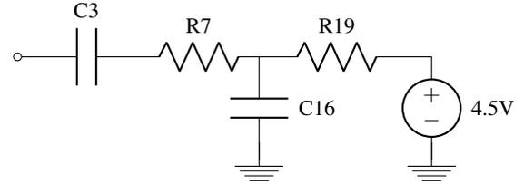
Figure 3: Klon Centaur Feed-Forward Network 1 Circuit
