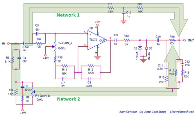
Figure 11: Circuit schematic for the gain stage from the Klon Centaur pedal, with the two Feed-Forward networks highlighted. Adapted from [2].
