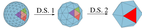
Figure 5: Downsampling layers based on the subdivision structure of the spherical meshes. The tensors in the previous layer, which are corresponding to a common triangle in the next layer, are merged to the tensor associated with the father triangle. These downsampling layers respect the spatial relations among the triangles.
