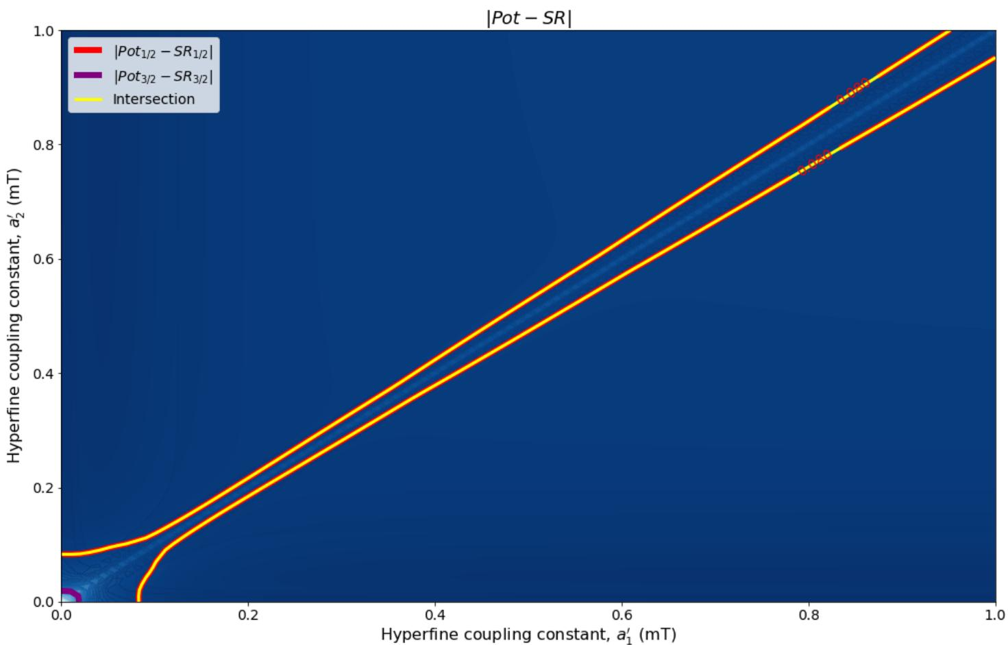
**Supplementary Figure S2.** The dependence of the two-xenon RPM model on changes in the hyperfine coupling constants  $a'_1$  and  $a'_2$  for  $a'_1, a'_2 \in [0, 1000] \mu\text{T}$ , using  $r = 1.0 \times 10^6 \text{ s}^{-1}$ ,  $B = 50 \mu\text{T}$ , and  $\tau = 4.9 \times 10^{-6} \text{ s}$ . The model can explain the experimentally derived<sup>6</sup> relative anesthetic potency of xenon where  $|Pot_{1/2} - SR_{1/2}| \leq 0.080$  and  $|Pot_{3/2} - SR_{3/2}| \leq 0.08$  intersect.
