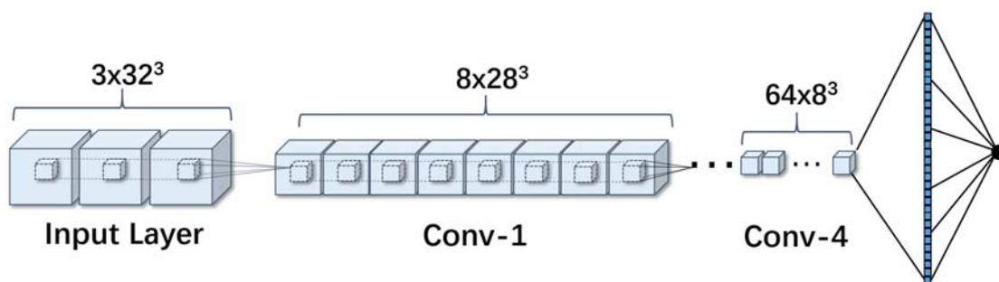
Figure 2. The architecture of the CNN network in this work.<sup>[26]</sup> Note that not all convolutional layers are shown due to space limitations. Each cube represents a 3D image. The input layer has three channels, similar to the RGB channels in 2D images. The output is a single score, indicating the likeness of the input structure to the native structure.
