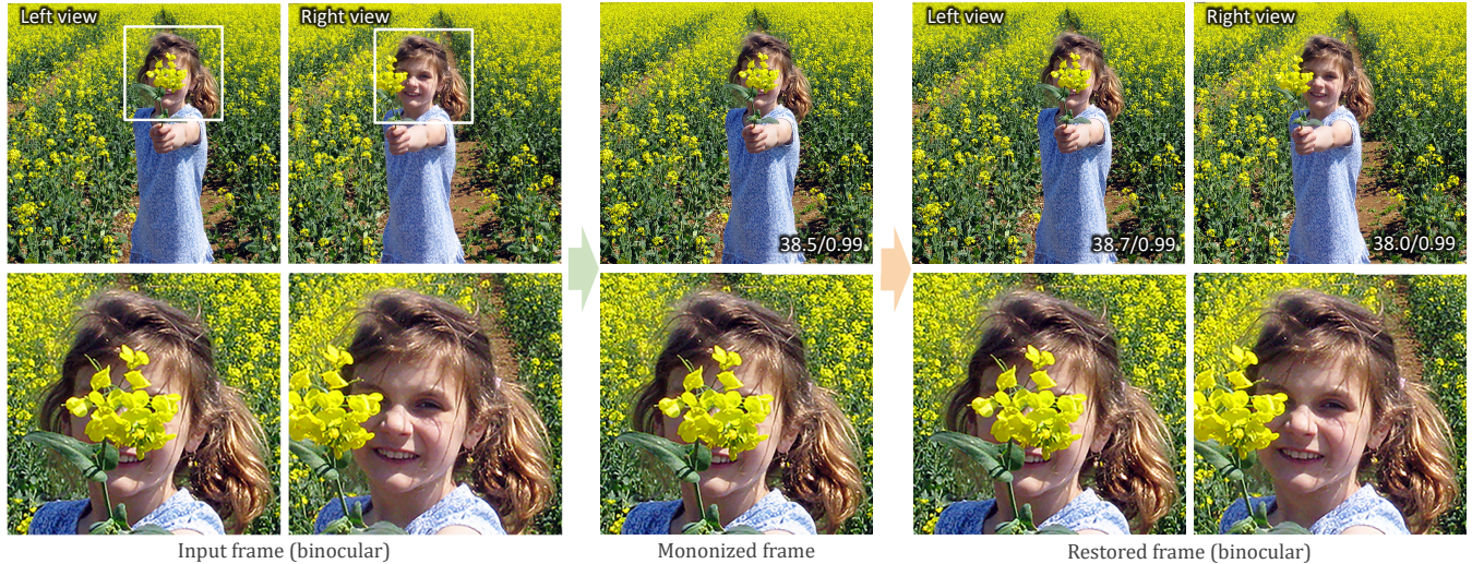
Fig. 1. Our method can effectively mono-nize a binocular video into a monocular video with the stereo information encoded in a nearly-imperceptible form. Note, the face of the little girl in the input right view (left); we can fuse it with the left view and encode (hide) it in the mononized frame (middle). Though the face is not observable in the mononized frame, we can restore it back in the restored binocular frame (right). We show PSNR/SSIM at the bottom of each result.
