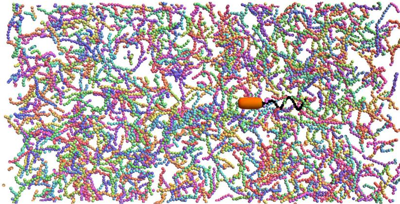
Figure 4: Sketch of a model bacterium swimming in a polymer solution consisting of bead-polymers and the background MPCD fluid (not shown).
