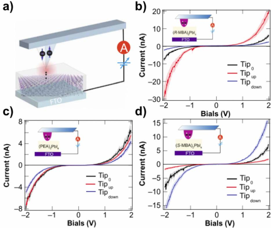
**Fig. 5:** (a) Experimental scheme for magnetic conductive atomic force microscopy (AFM) measurement of chiral perovskite thin films. (b)-(d) Current–voltage traces collected for thin films of lead–iodide perovskites containing chiral R-methylbenzylammonium, achiral phenylmethylamine, and chiral S-methylbenzylammonium, respectively, as a function of tip-magnetization orientation. Reproduced with permission from Ref. 40. Copyright 2019 by the American Association for the Advancement of Science.
