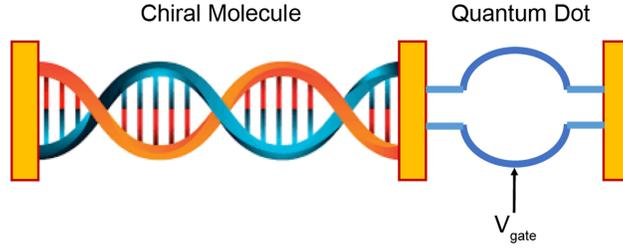
**Fig. 20:** A schematic illustration of a ‘super chiral molecule’ – a coupled chiral-molecule/quantum-dot hybrid structure, for controlling and manipulating spin polarization and entanglement. The gate voltage is applied to change the QD structure for controlling spin polarization.
