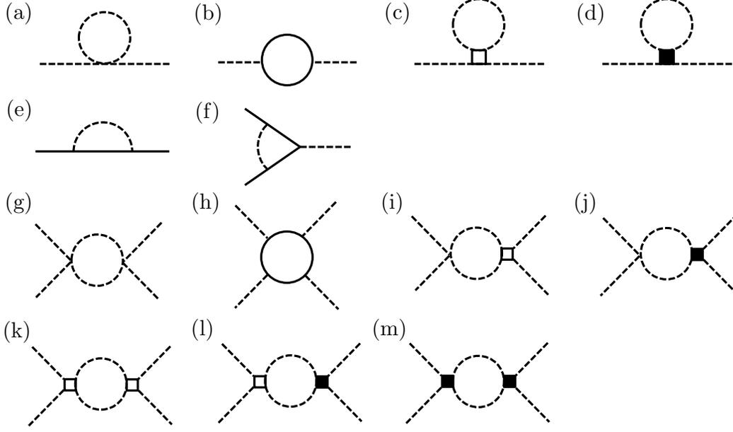
FIG. 3. Schematic one-loop Feynman diagrams for the random-mass GNY models. Renormalization of (a,b,c,d) the boson two-point function; (e) the fermion two-point function; (f) the Yukawa vertex  $h$ ; (g,h,i,j) the boson self-interaction vertex  $\lambda^2$ ; (i,k,l,m) the short-range correlated disorder vertex  $\Delta$ ; and (j,l,m) the long-range correlated disorder vertex  $v$ .
