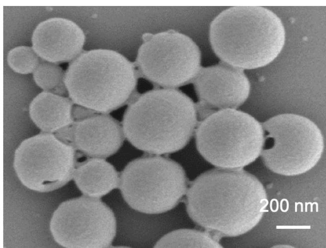
**Figure 2.** Scanning electron micrograph (SEM, Ultra 55, 10 keV) of a small cluster of primary nanoparticles. The core-shell structure is not thermally stable under the exposure to high energy density, such as a focused electron beam in higher magnification and the nanoparticle will partially melt to present irregular shape.
