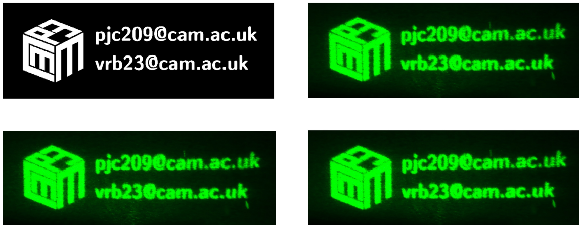
Figure 4: Target image (top left) with 24 sub-frames shown on a 1024 \times 1024 pixel binary phase projector with a ball lens. The top half of the holographic replay fields are shown for 24 frames of OSPR (bottom left), 24 frames of STTM (top right) and 4 sets of 6 frames of STTM (bottom right). The STTM and hybrid frames are generated in < 5\% and < 20\% respectively of the time with little visual difference. Captured using a Canon 5D Mark III with a 24-105mm lens and a 1/60 second exposure.
