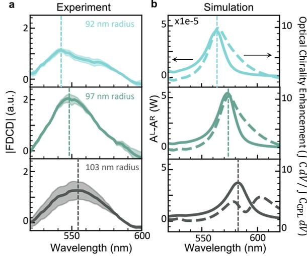
Figure 4: a) Normalized FDCD signal from dye-dsDNA on  $r=92-103\text{nm}$  arrays (details in SI). Vertical lines mark spectra maxima, illustrating red-shift, shaded region represents standard error. b) Simulated  $\Delta A$  from 10nm chiral layer on disk surface (left axis, solid) against integrated  $C/C_{\text{CPL}}$  (right axis, dotted). Vertical lines mark  $\Delta A$  maxima.
