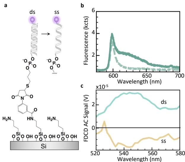
Figure 3: a) Functionalization scheme and de-hybridization on substrate b) Fluorescence of dye-functionalized 92-nm-radius array (solid) vs dye-less (dotted) c) FDCD sign reversal from dye-dsDNA to dye-ssDNA
