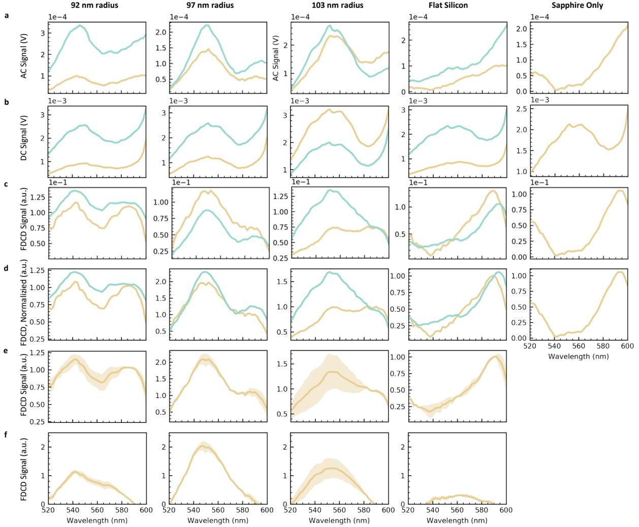
Figure S 9: Workflow of data analysis from raw data to data in main text a) AC Signal as calculated by  $-V_{RMS} * \sin(\theta)$  b) DC signal,  $V_{DC}$  c) FDCD signal as calculated by  $-V_{RMS} * \sin(\theta)/V_{DC}$  d) FDCD signal normalized by value of spectrum at 590 nm e) Averaged FDCD spectrum plotted with standard error f) Averaged spectrum with sapphire background subtracted.
