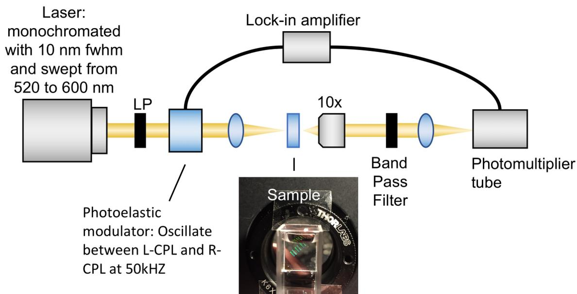
Figure S 3: Schematic of table-top fluorescence detected circular dichroism spectrometer
