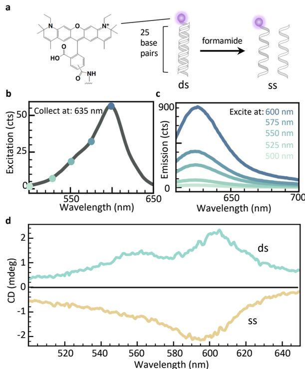
Figure 2: a) Structure of Atto<sup>TM</sup>590 dye functionalized to 5'-end of DNA & de-hybridization scheme b) Excitation spectrum of dye-dsDNA in PBS c) Emission spectra of dye-dsDNA in PBS d) CD of dye-dsDNA & dye-ssDNA in PBS, 30 $\mu\text{M}$ .
