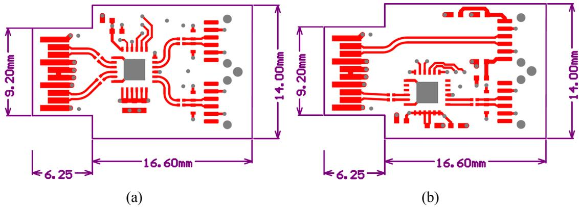
**Figure 1.** PCB design of MTx+ (a) and MTRx+ (b).
