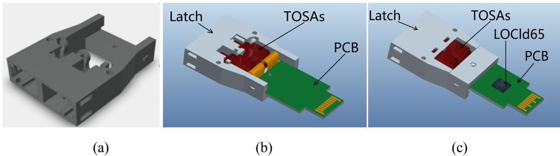
**Figure 2.** Bottom view of a latch (a), bottom view (b) and top view (c) of an MTx+ module.
