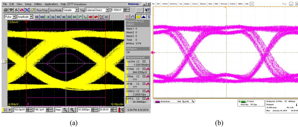
**Figure 6.** Eye diagrams of MTx+ (a) and MTRx+ (b).
