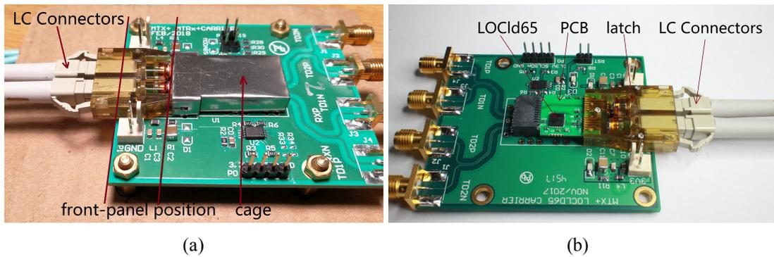
**Figure 4.** Pictures of panel-mount (a) and board-mount (b) MTx+ plugged in the motherboard.
