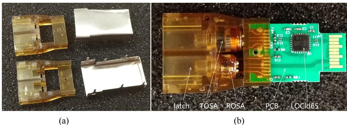
**Figure 3.** Pictures of latches and cages (a) and an MTRx+ module (b).
