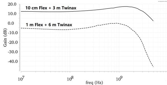
Figure 12: AC Response of the recovered signals
