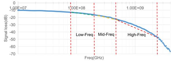
Figure 11: Simulation of Cable Loss based on 1-m flex model and 6-m Twinax model in series
