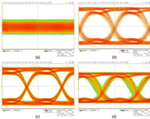
Figure 6: Eye diagrams (a) after the 6m Twinax cable and before the GBCR, (b) after the GBCR (CDR is off) (c), after the GBCR (CDR is on) (d) after the GBCR, one example with obvious DC offset
