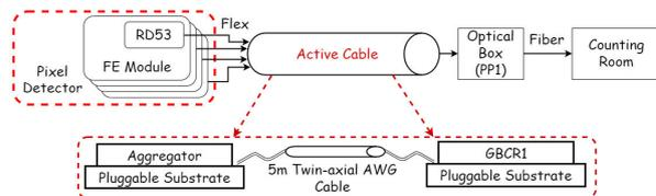
Figure 1: The original ITk Readout System Plan
