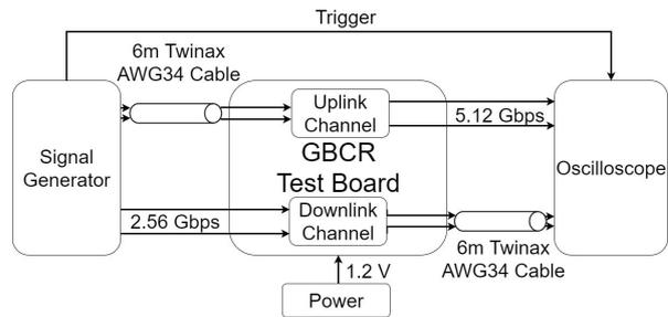
Figure 5: Block Diagram of GBCR1 Test Bench
