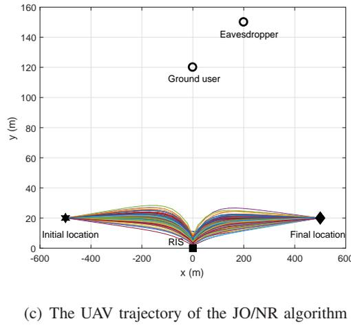
Fig. 3. UAV trajectories by using different algorithms with  $T = 124$  s,  $\delta_a^2 = 0.5$ ,  $\bar{P} = \bar{G} = 20$  dBm, and  $w = 0.5$
