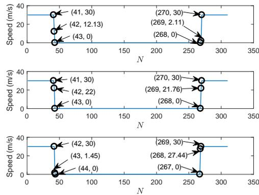
Fig. 4. Upper figure: UAV speed (m/s) versus  $N$  for the JO algorithm; middle figure: UAV speed (m/s) versus  $N$  for the JO/NR algorithm; lower figure: UAV speed (m/s) versus  $N$  for JO/NPB algorithm. The system parameters are set as  $T = 124$  s,  $\delta_a^2 = 0.5$ ,  $\bar{P} = \bar{G} = 20$  dBm, and  $w = 0.5$ .
