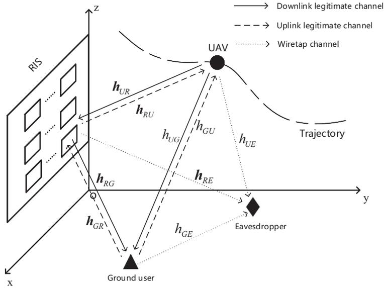
Fig. 1. A RIS-assisted UAV secure communication system<sup>3</sup>.
