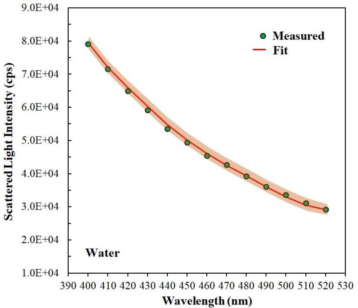
**Figure 8.** Plot showing the peak height intensities of scattered light measured for pure water for different incident light wavelengths and the best fit line obtained using equation 4.1 for the data in the wavelength range of 370 – 510 nm. The goodness of fit was verified by calculating the  $R^2$  parameter ( $R^2 = 0.9955$ ).
