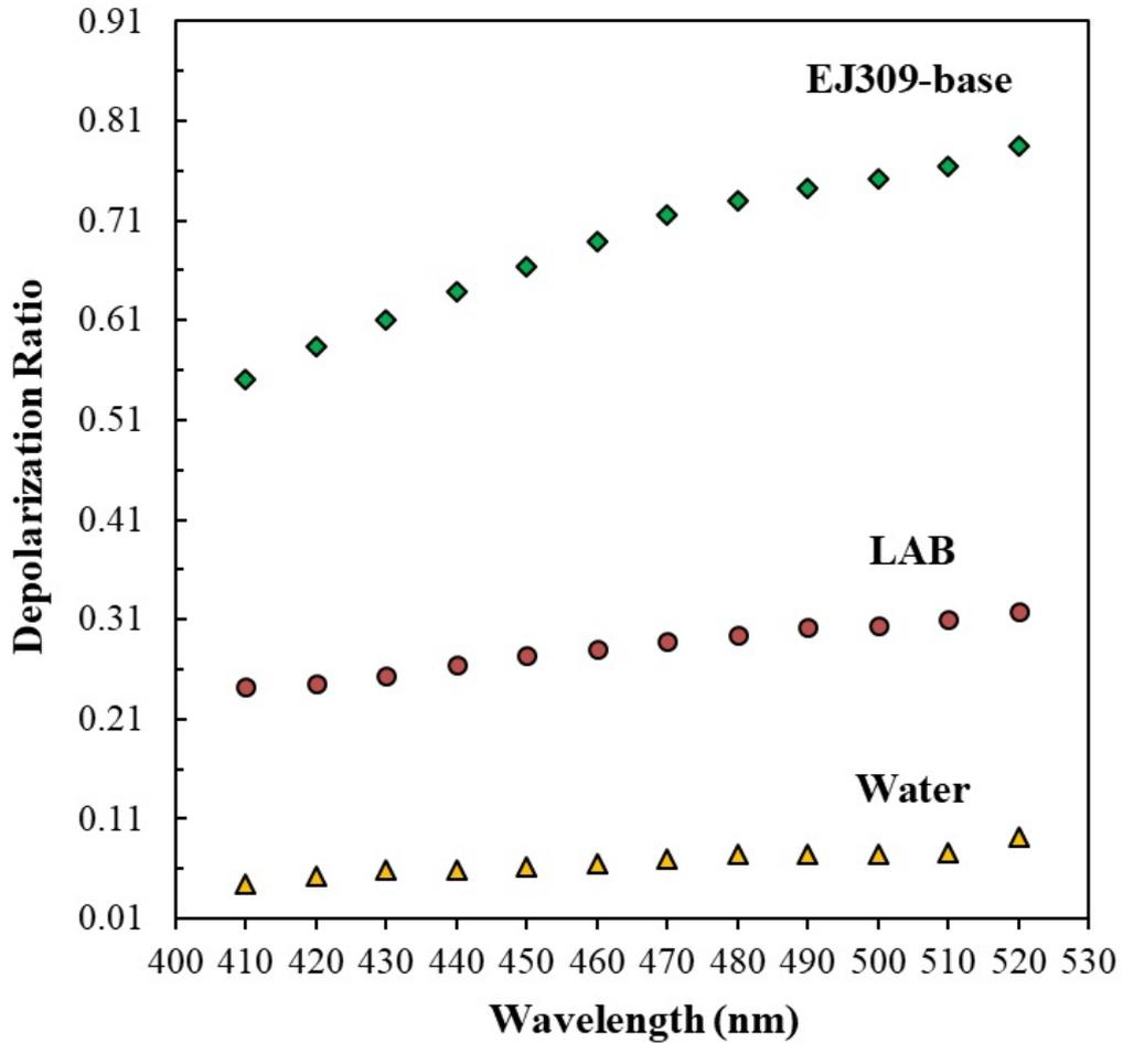
**Figure 5.** Depolarization ratios over a range of wavelengths for the three pure liquid samples. (data in the literatures are only available at  $\lambda=430\text{nm}$ :  $0.29\pm 0.03$ ,  $0.31\pm 0.03$ ,  $0.33\pm 0.03$  for 3 different types of LABs)
