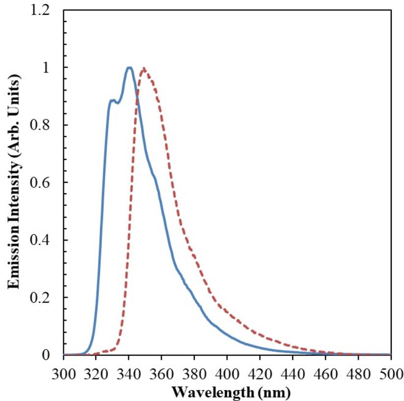
**Figure 1.** Emission spectra of pure LAB (solid) and EJ309-base (dash) with excitation  $\lambda = 260\text{nm}$ .
