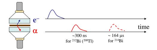
Figure 26: Principle of the BiPo detectors to identify BiPo events: electron and alpha emissions from the sample are detected in opposite scintillators following a particular time sequence (courtesy of the SuperNEMO collaboration).
