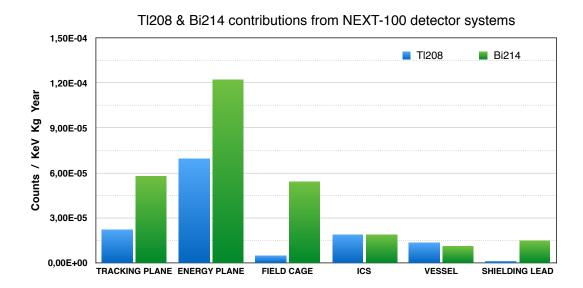
Figure 19: Background budget for NEXT-100 after event selection from  $^{214}$ Bi (right columns) and  $^{208}$ Tl (left columns) emissions coming from the different detector subsystems (as presented in [262]).
