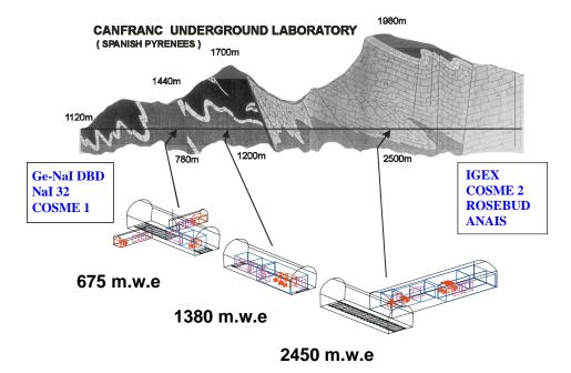
Figure 3: Mountain profile and location along the railway tunnel of the first facilities of the LSC, used before the construction of the present LAB2400. The corresponding rock overburden and the main experiments carried out there are also indicated. The facilities at 780 m and 2500 m from the Spanish entrance of the train tunnel (now referred as LAB780 and LAB2500, respectively, see also Fig. 4) are still in use.
