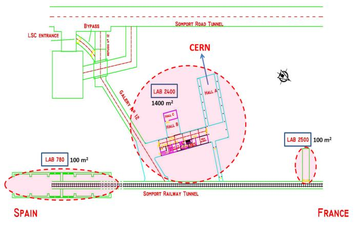
Figure 4: Layout of the present underground facilities at LSC. The main infrastructures, LAB2400 with halls A and B and LAB2500, are located between the railway and road tunnels (courtesy of LSC).
