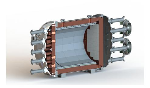
Figure 18: Cross-section view of the design of the NEXT-100 detector (courtesy of the NEXT collaboration). A stainless steel pressure vessel houses the electric-field cage and the two sensor planes (energy plane and tracking plane) located at opposite ends of the chamber. The fiducial region is a cylinder of 1050 mm diameter and 1300 mm length (defining  $1.27 \text{ m}^3$  of fiducial volume). The active volume is shielded from external radiation by at least 12 cm of copper in all directions.
