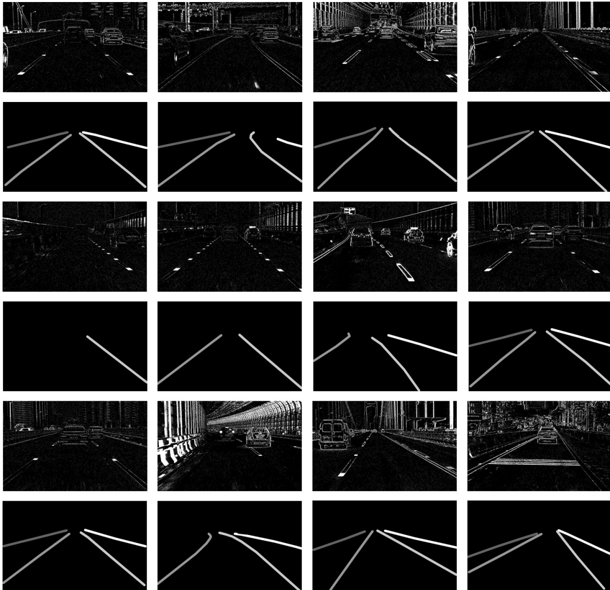
Fig. 4. Samples of DVS images and labels in DET. First rows show various line types, including single dotted line, single solid line, parallel dotted line, parallel solid line and dotted line. Middle rows show various lane number, from 1 to 4. Last rows show various traffic scenes, urban, tunnel, bridge and overpass.
