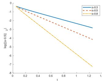
FIGURE 5.5. Time evolution of  $\log \left( \|u - \frac{1}{|\Omega|} \int_{\Omega} u_0\|_{L^2(\Omega)} \right) = \log \left( \|u - 0.5\|_{L^2(\Omega)} \right)$  in Example 5.5. The linear relation between both quantities agrees with the exponential decay predicted in [24].
