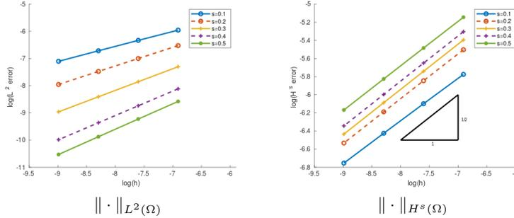
FIGURE 5.1. The  $L^2(\Omega)$  and  $H^s(\Omega)$  errors in logarithmic scale for Example 5.2, using several values of  $s$ . In these experiments we used uniform meshes with  $h = 1/1000, 1/2000, 1/4000, 1/8000$ , and  $H = 1.2$ . The observed order of convergence is approximately  $s + 1/2$  and  $1/2$  in the  $L^2(\Omega)$  and  $H^s(\Omega)$  norms, respectively.
