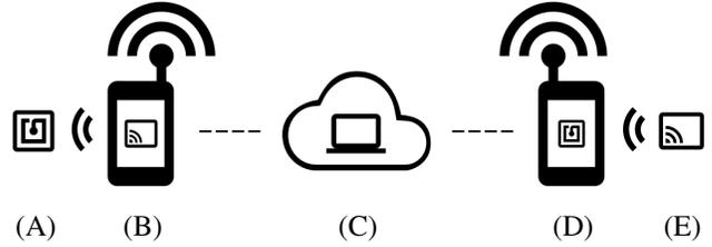
Figure 3: NFCGate relay setup with external server.
