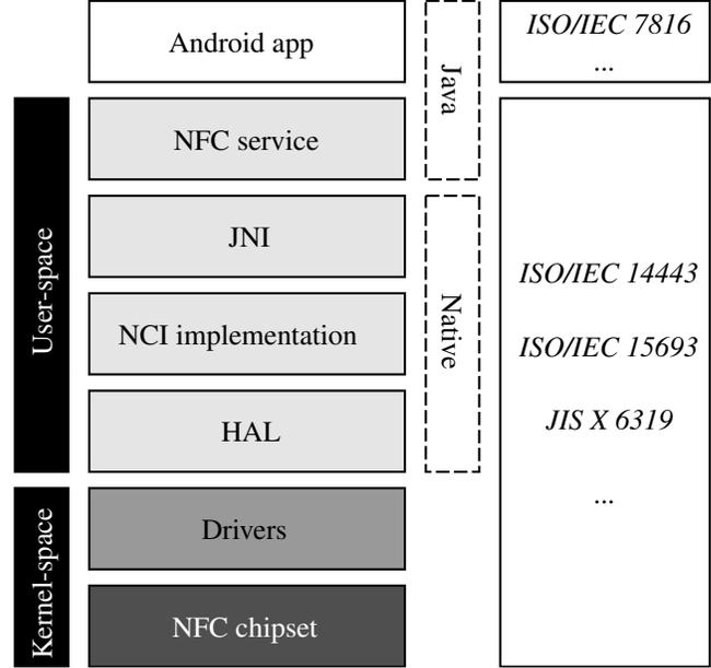
Figure 1: Architecture of the Android NFC stack.
