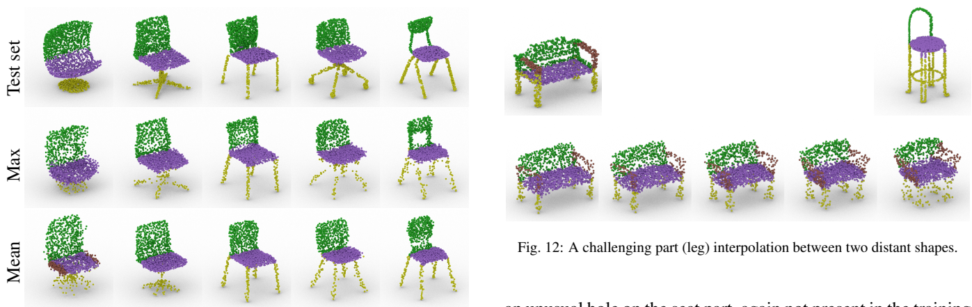
Fig. 11: Reconstruction comparison between models using max and mean pooling.
