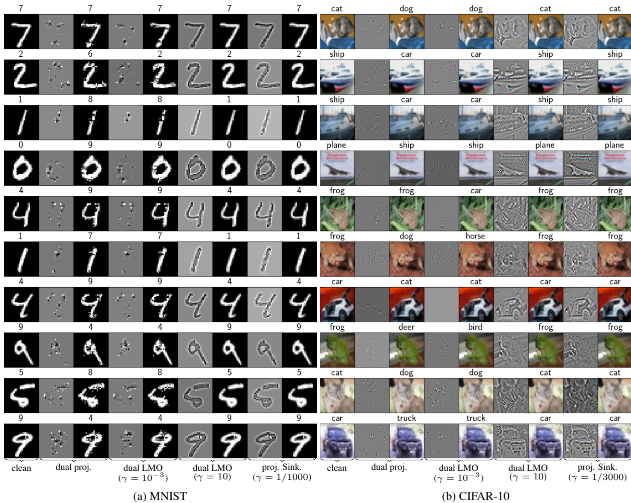
Figure 9: Comparison of Wasserstein adversarial examples and Wasserstein perturbations generated by different attacks on MNIST ( \epsilon = 0.2 ) and CIFAR-10 ( \epsilon = 0.002 ). Predicted labels are shown on the top of images. Perturbations are scaled linearly to [0, 1] for visualization.
